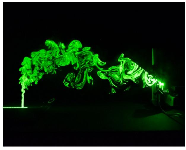
Demonstration of air flow through ceiling penetration at the mean ceiling-roof cavity pressure difference of 1.2 Pa using smoke and LED light.
