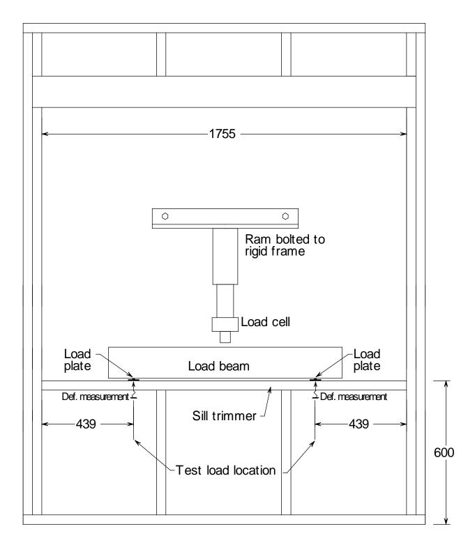
Figure 2. Elevation of test setup – before support system is installed.
