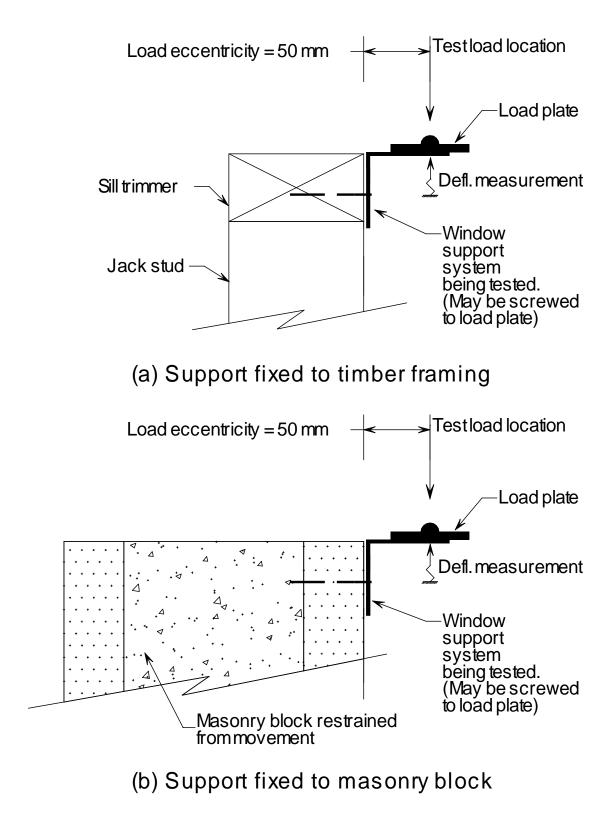
Figure 1. Cross section of test loading of window frame.
