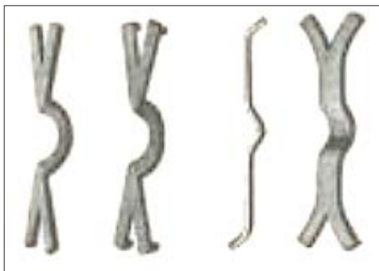
(a) Cast iron (left 2) and wrought iron (right 2) ties (reproduced from Hamilton, 1958)
