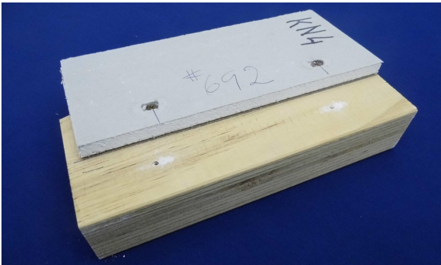
Figure 1. Plasterboard slip testing specimen
