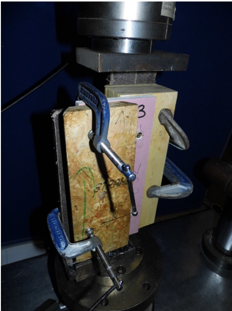
Figure 2. Assembled slip test specimen following testing.
