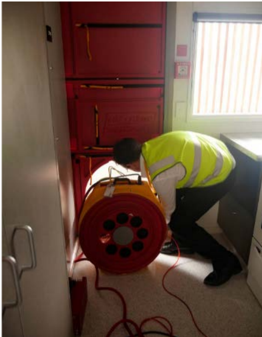
Figure 30. BRANZ scientist installing blower unit in the base of entry door.
