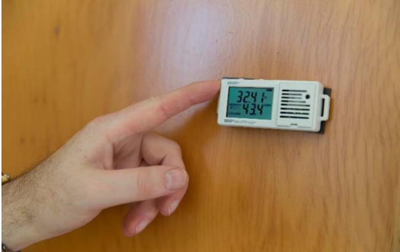
Figure 20. Temperature and relative humidity sensor/logger on kitchen door. (Photography: WCC)
