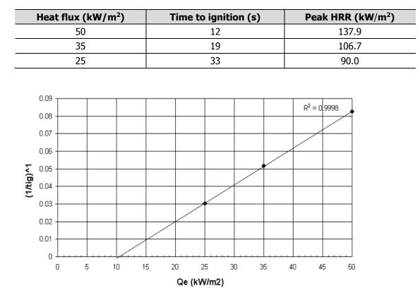
Table 9. Summary of data from cone calorimeter tests.
