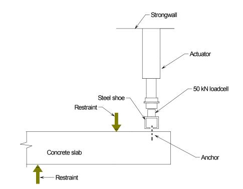
Figure 6. Plan view of the test set-up.
