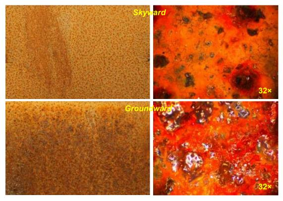
Figure 36. Typical morphology of mild steel coupons after one year exposure at Tiwai Point
