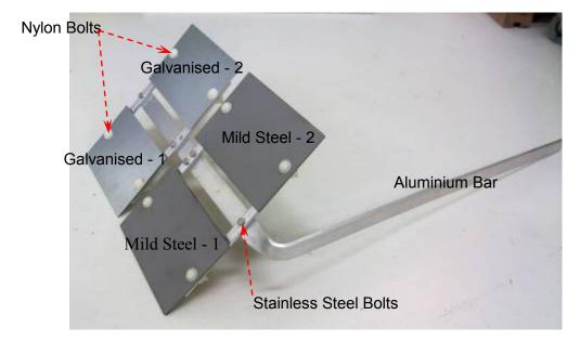
Figure 3. Exposure rack carrying mild steel and hot dip galvanised steel coupons used in the present study
