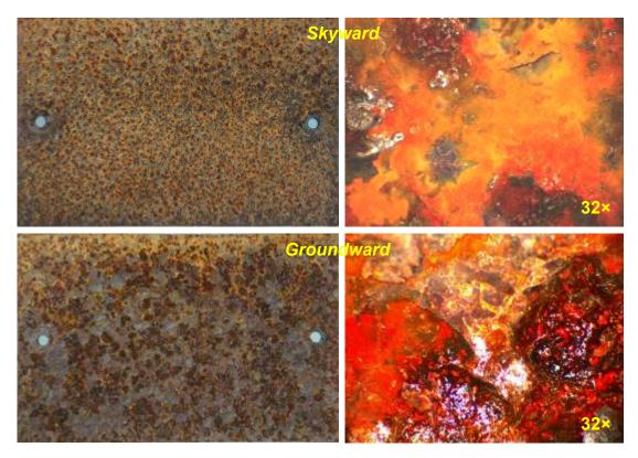
Figure 30. Typical morphology of mild steel coupons after one year exposure at Auckland Airport
