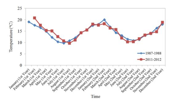
Figure A41. Comparison of ambient temperatures in the periods of 1987 – 1988 and 2011 - 2012 for Ardmore
