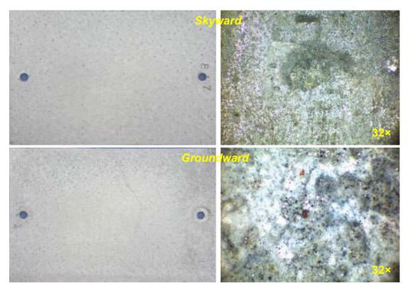
Figure 39. Typical morphology of hot dip galvanised steel coupons after one year exposure at Tiwai Point
