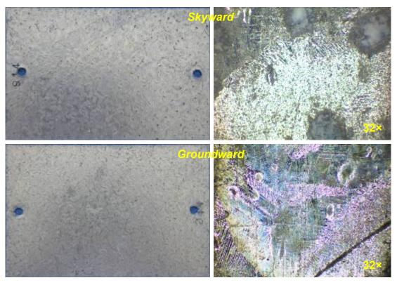
Figure 42. Typical morphology of hot dip galvanised steel coupons after one year exposure at Forbury, Dunedin
