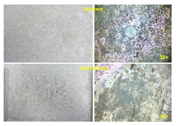
Figure 35. Typical morphology of hot dip galvanised steel coupons after one year exposure at Gracefield, Lower Hutt
