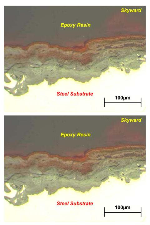
Figure 28. Cross-sectional morphology of mild steel coupons after one year exposure at Waitoki
