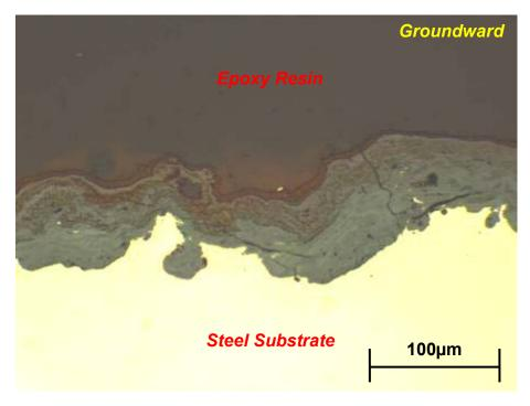
Figure 34. Cross-sectional morphology of mild steel coupons after one year exposure at Gracefield, Lower Hutt
