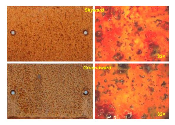
Figure 27. Typical morphology of mild steel coupons after one year exposure at Waitoki
