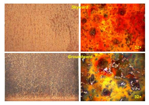
Figure 33. Typical morphology of mild steel coupons after one year exposure at Gracefield, Lower Hutt
