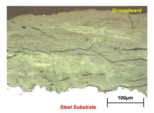
Figure 31. Cross-sectional morphology of mild steel coupons after one year exposure at Auckland Airport
