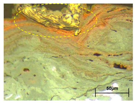
Figure 38. Inclusions of unknown composition found on the groundward face of the mild steel samples exposed at Tiwai Point
