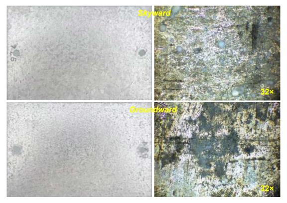
Figure 29. Typical morphology of hot dip galvanised steel coupons after one year exposure at Waitoki
