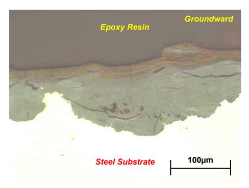
Figure 37. Cross-sectional morphology of mild steel coupons after one year exposure at Tiwai Point
