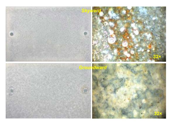
Figure 32. Typical morphology of hot dip galvanised steel coupons after one year exposure at Auckland Airport
