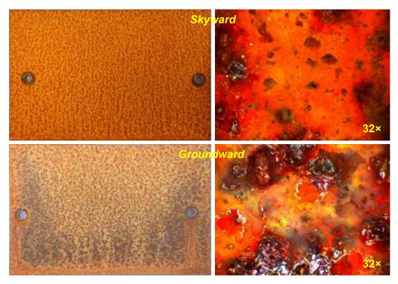
Figure 40. Typical morphology of mild steel coupons after one year exposure at Forbury, Dunedin
