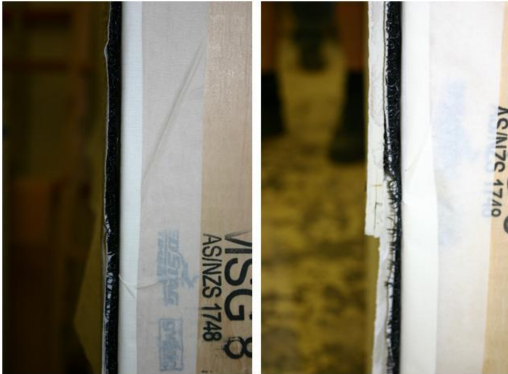
Figure A.11 Compression of Drainage Product after Cladding is Applied
