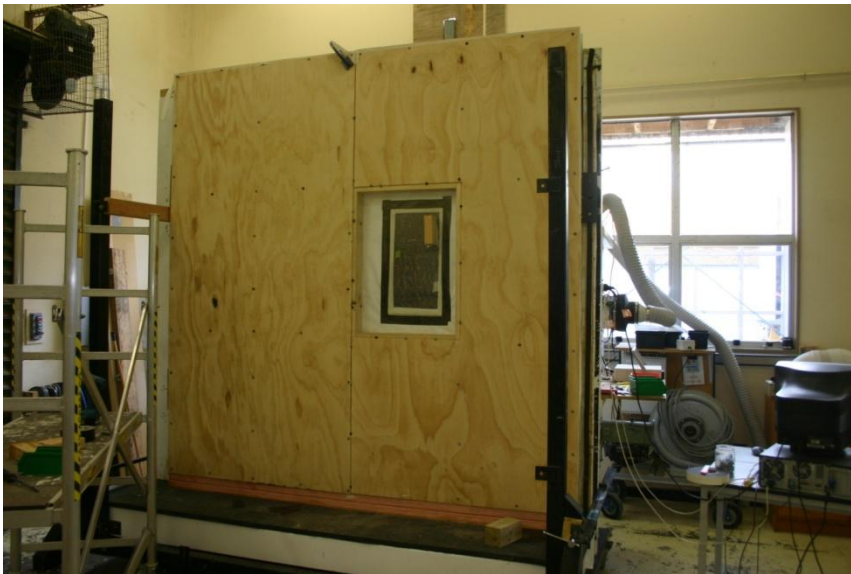
Figure A.12 Perspex Panels in Line with Underlay and Plywood Interior Linings
