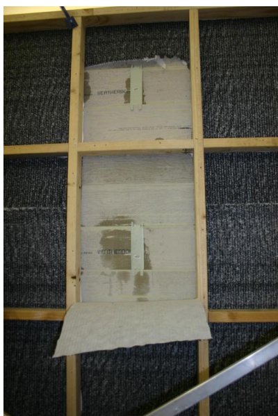
Figure A.13 Water Penetration Through Boards
