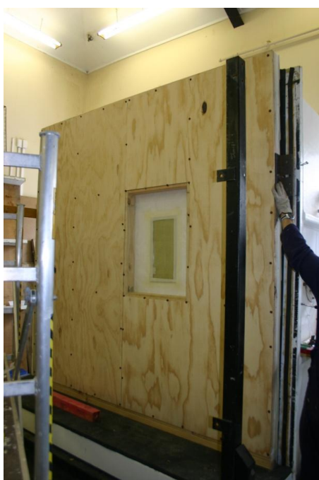
Figure A.9 Perspex Panels in Line with Underlay and Plywood Interior Linings
