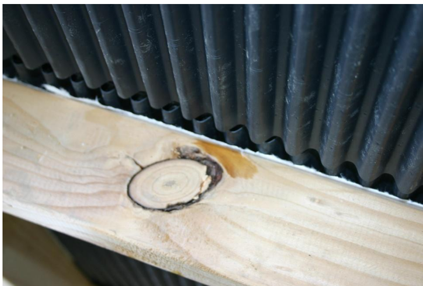
Figure A.17 Frame Wetting During the Wetwall Test Due to Product Not Lapping
