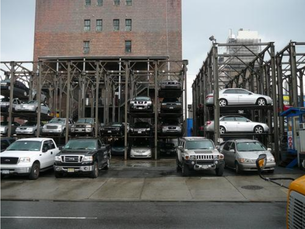
Figure 44: Outdoor stacking four-vehicles high in New York City
