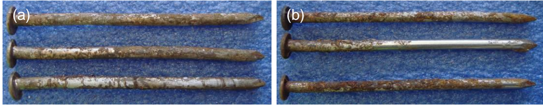
Figure 20. Surface morphologies of mild steel nails embedded into the H4 CuAz (a) and H4 ACQ (b) treated timber top surfaces.
