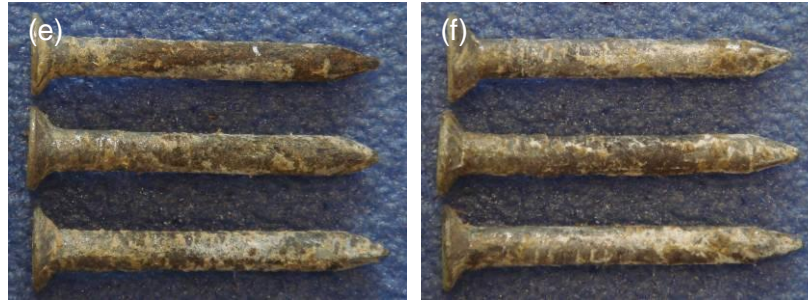
Figure 16. Surface morphologies of hot dip galvanised nails inserted into timber blocks from the top: (a) untreated, (b) H3 CCA, (c) H3 CuAz, (d) H4 CuAz, (e) H3 ACQ and (f) H4 ACQ.
