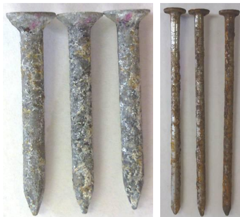
Figure 10. Surface morphologies of the nails retrieved from ACQ treated timbers (nails inserted into top surface of the timber block).
