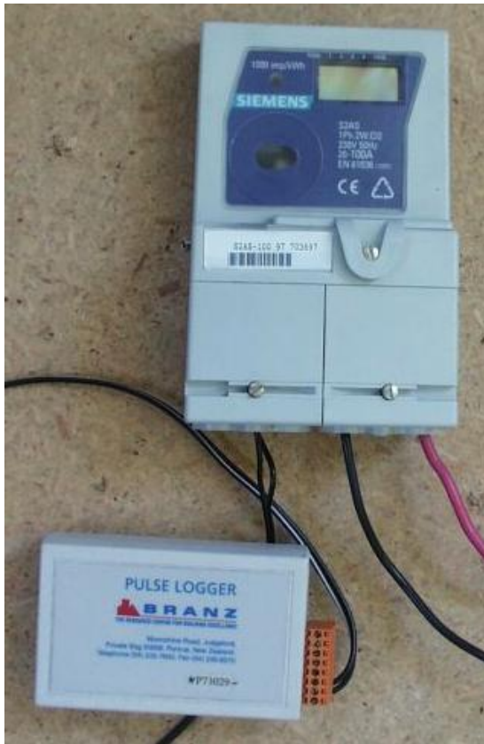
Figure 5. A Siemens S2AS electricity meter with a BRANZ pulse logger
