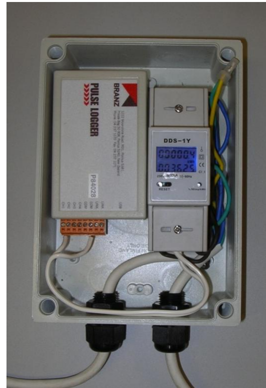
Figure 6. A DDS1Y DIN rail electricity meter alongside a BRANZ pulse logger
