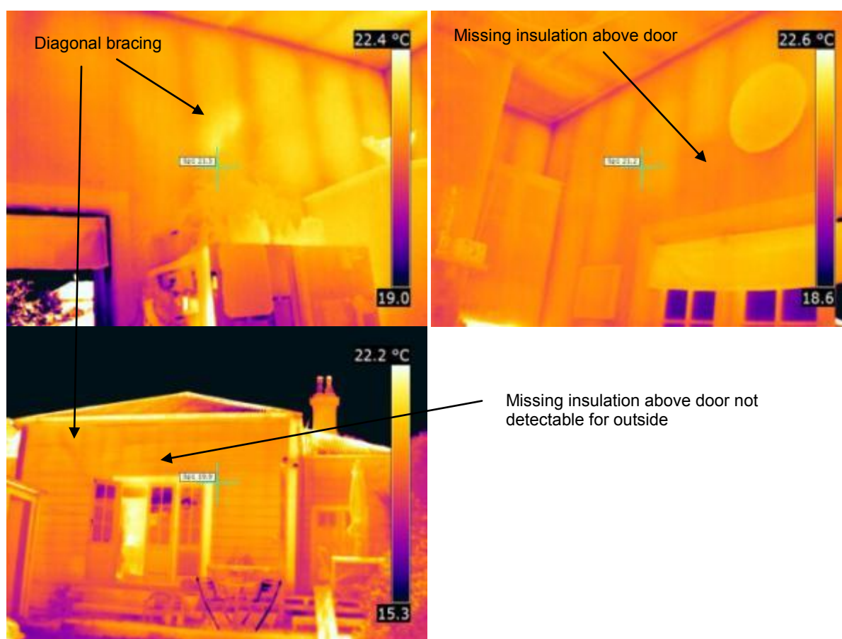
Figure 6: Bevel-backed weatherboard-clad wall imaged from both the interior and exterior of a house.
