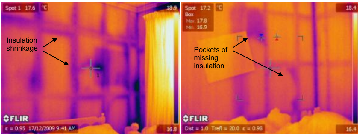
Figure 10: An example (left image) of insulation shrinkage creating gaps against framing and an example (right image) with little to no shrinkage but with missing pockets of insulation.
