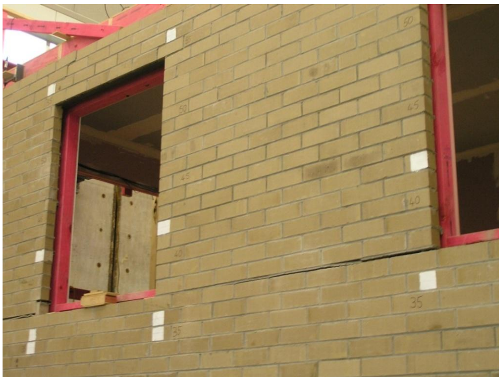
Figure 55. Cracking in Side 1 veneer at Panel B at peak pull in Stage D
