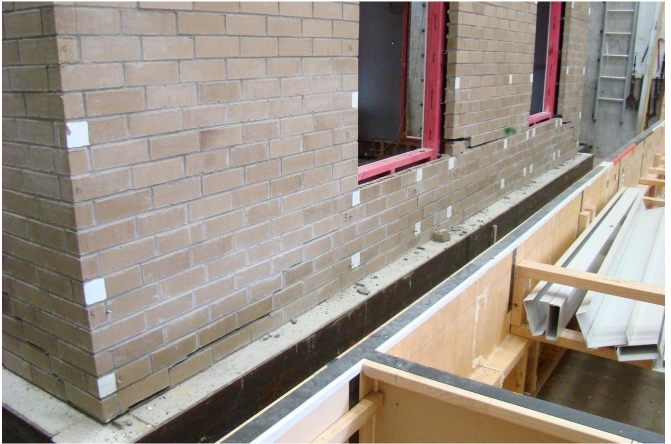
Figure 103. Cracking in Side 2 bottom spandrel at peak pull in Stage I
