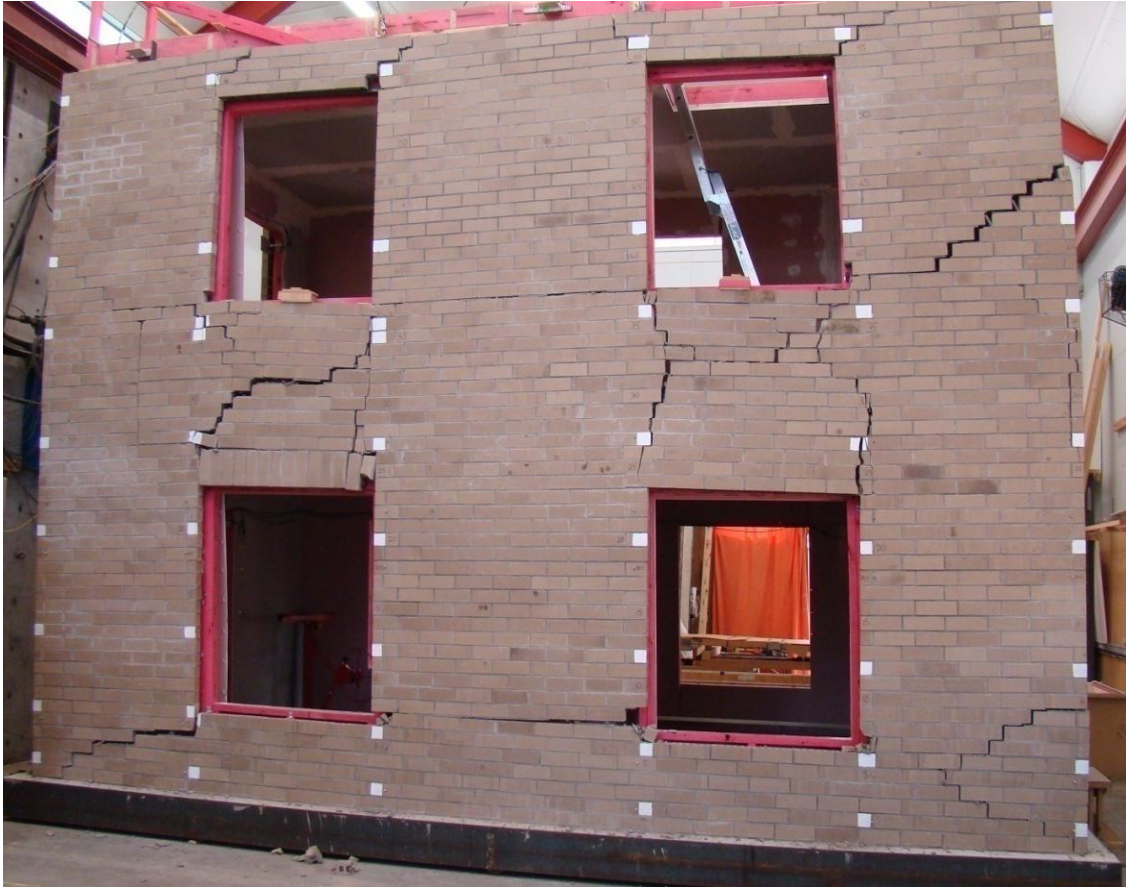
Figure 99. Cracking in Side 1 veneer at peak pull in Stage I
