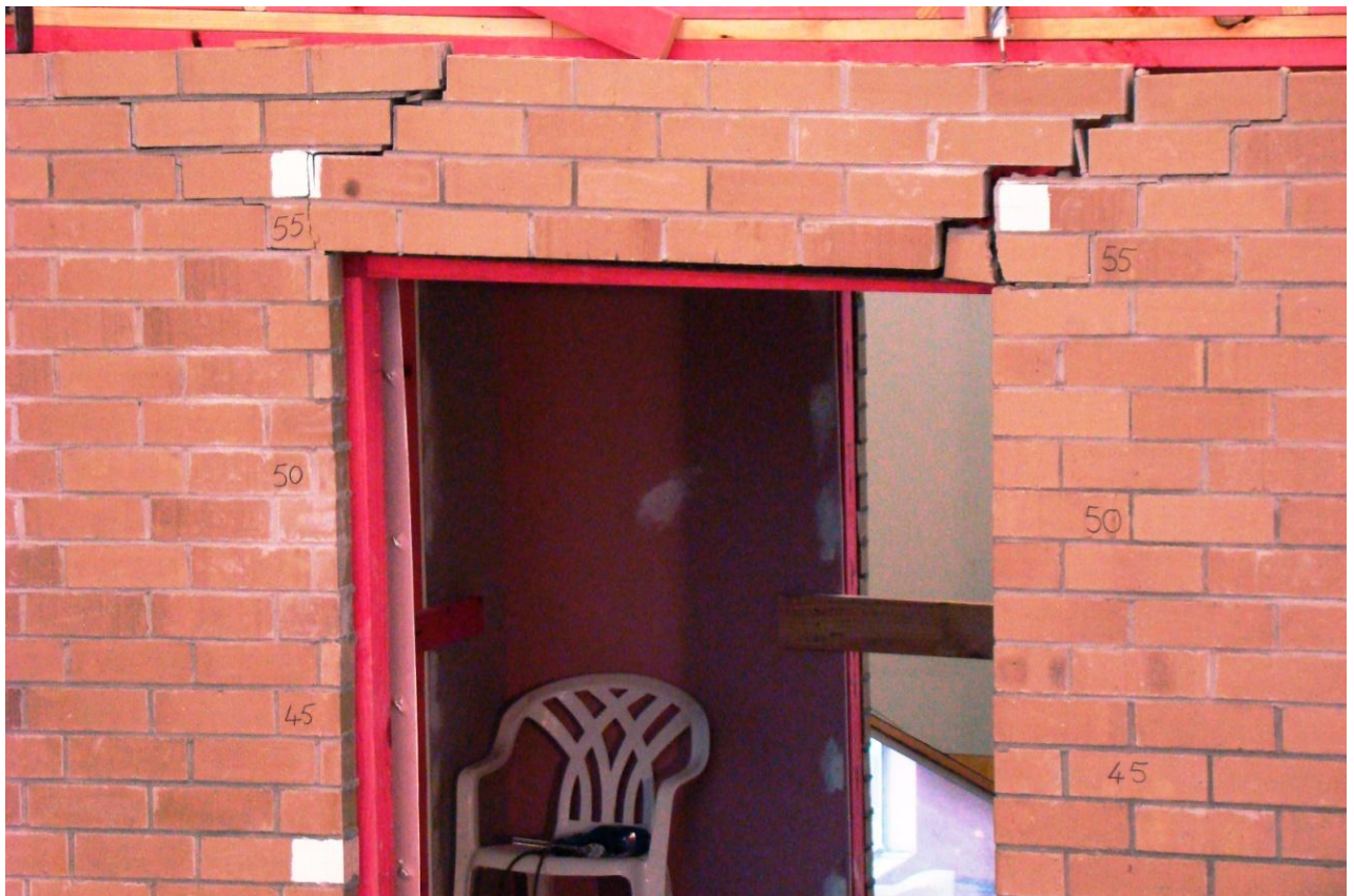
Figure 54. Lintel cracking above Side 1 Window S1C at peak pull in Stage G
