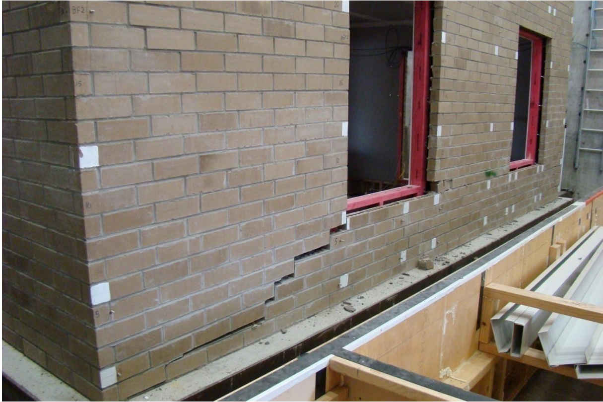
Figure 101. Cracking in Side 2 bottom spandrel at peak push in Stage I
