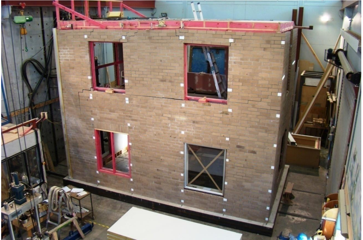
Figure 75. Cracking in Side 1 veneer at peak pull in Stage F
