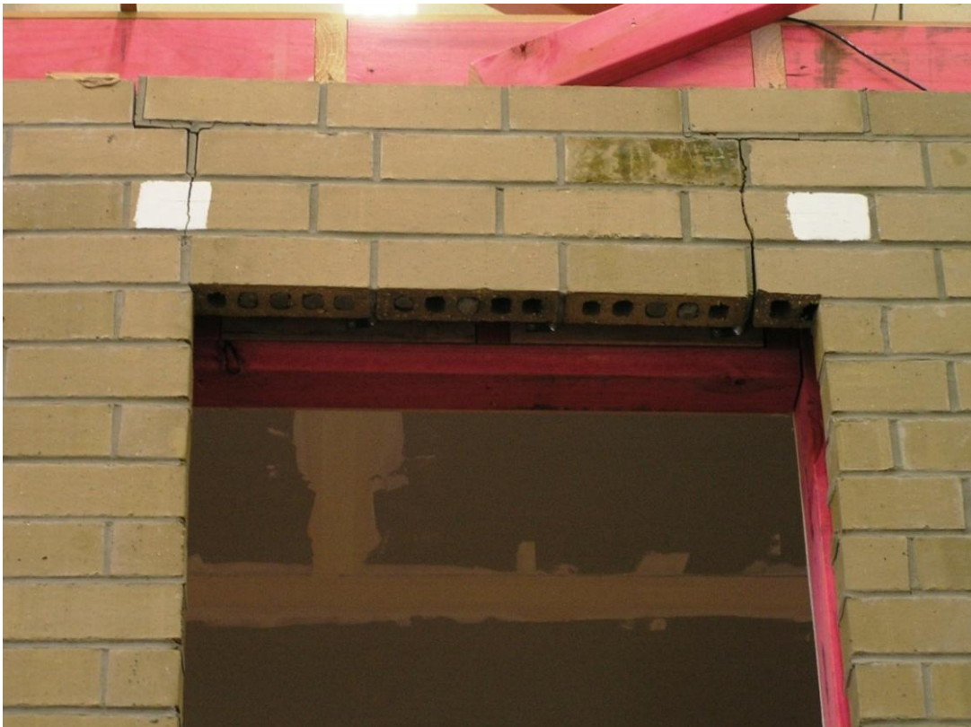
Figure 50. Lintel cracking above Side 2 Window S2C at peak push in Stage D
