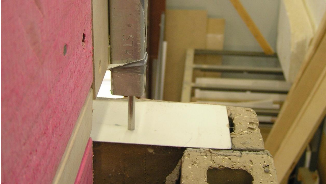
Figure 29. Measurement of vertical displacement of LTF relative to the veneer
