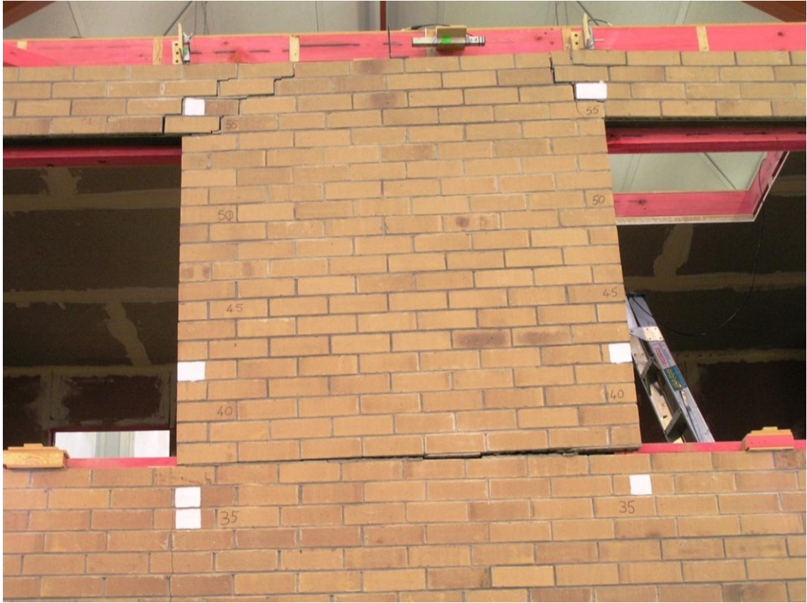
Figure 77. Cracking in Side 1 veneer at Panel B at Peak pull in Stage F
