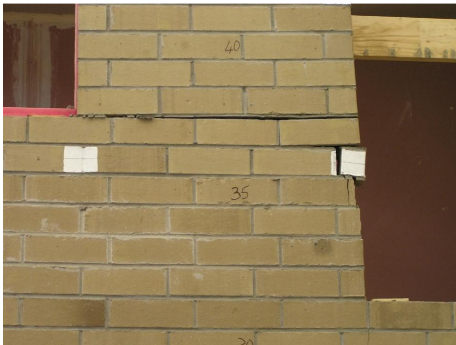
Figure 88. Cracking in Side 2 upper-storey veneer at Panel G at peak push in Stage F
