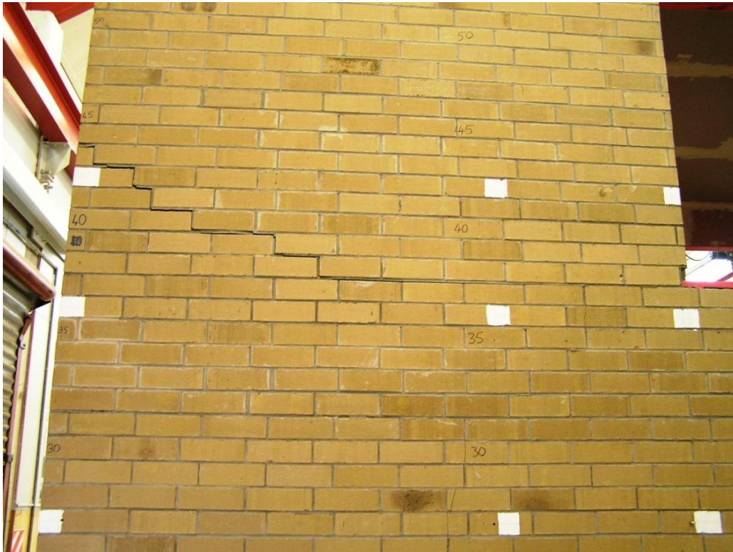
Figure 67. Cracking in Side 2 upper-storey veneer at Panel F at peak pull in Stage E
