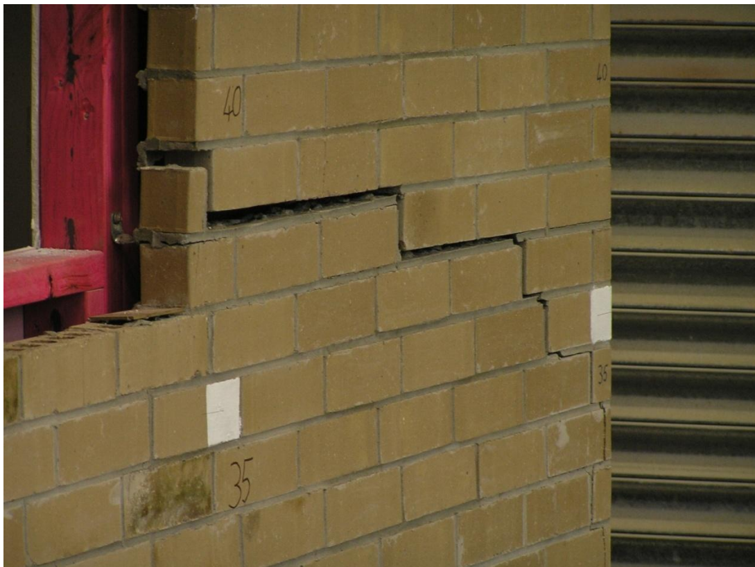
Figure 82. Cracking in Side 1 veneer at Panel C top window at peak push in Stage F
