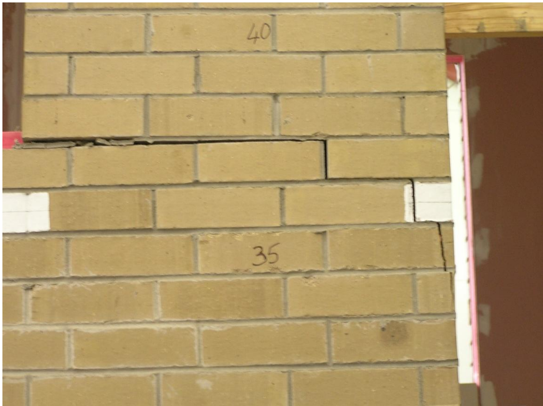
Figure 70. Cracking in Side 2 upper-storey veneer at Panel G at peak pull in Stage E
