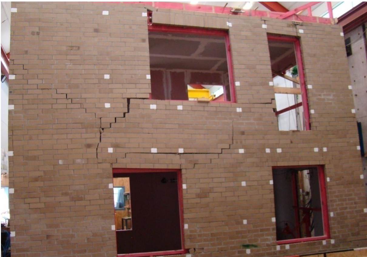
Figure 100. Cracking in Side 2 veneer at peak push in Stage I
