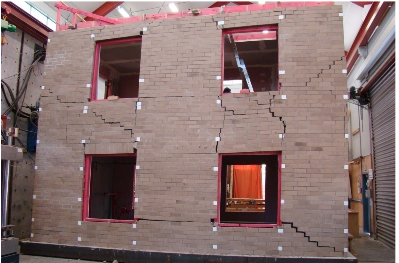
Figure 98. Cracking in Side 1 veneer at peak push in Stage I
