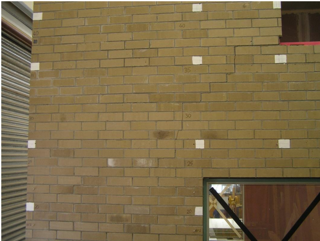
Figure 71. Residual cracking Side 1 Panel F veneer at zero load after Stage E cycling
