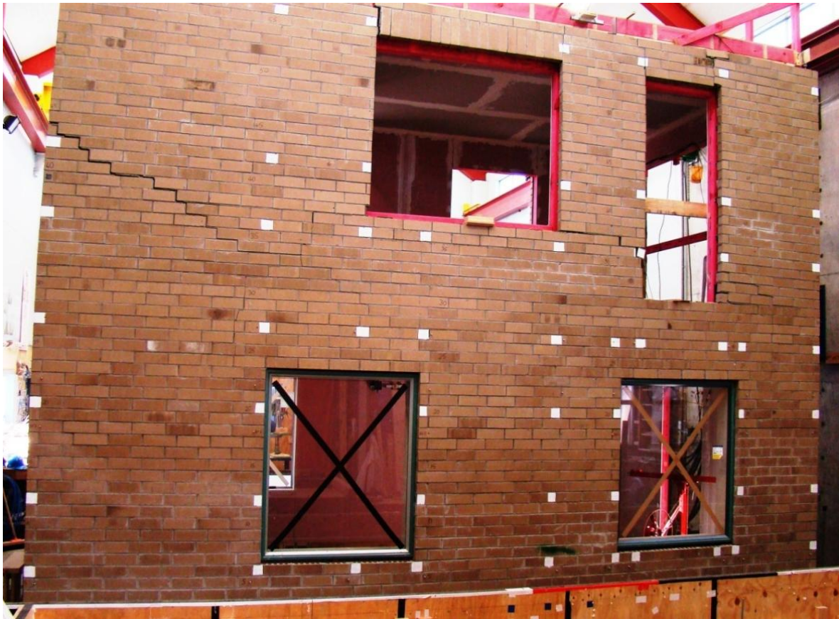
Figure 85. Cracking in Side 2 veneer at peak pull in Stage F
