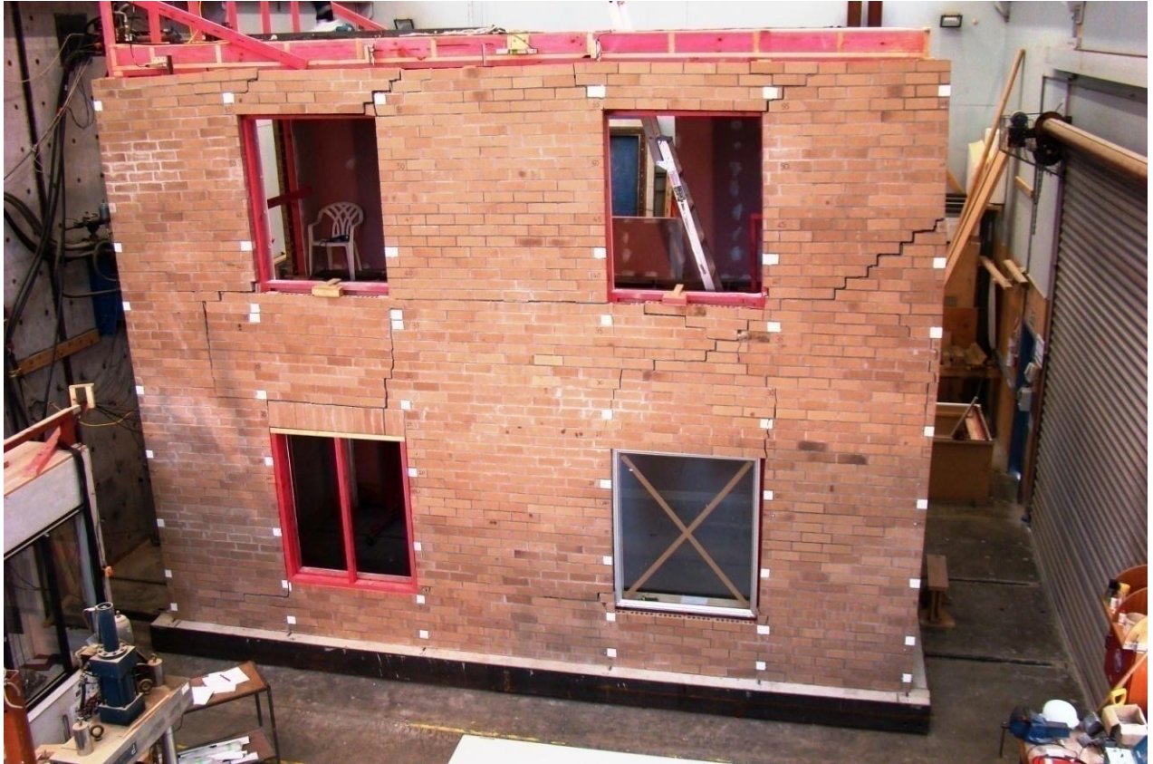
Figure 91. Cracking in Side 1 veneer at peak pull in Stage G
