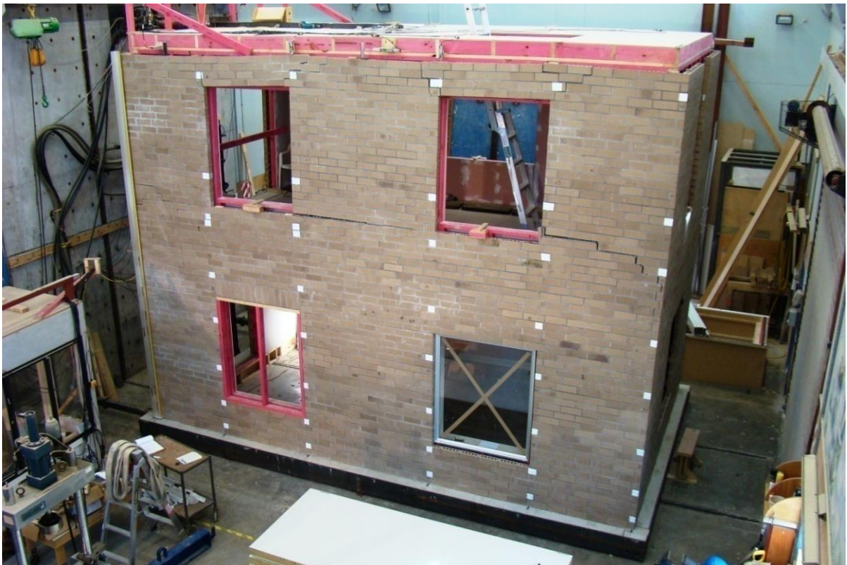
Figure 74. Cracking in Side 1 veneer at peak push in Stage F
