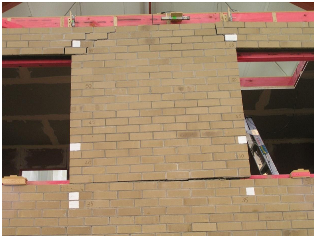
Figure 80. Cracking in Side 1 veneer at Panel B at peak pull in Stage F
