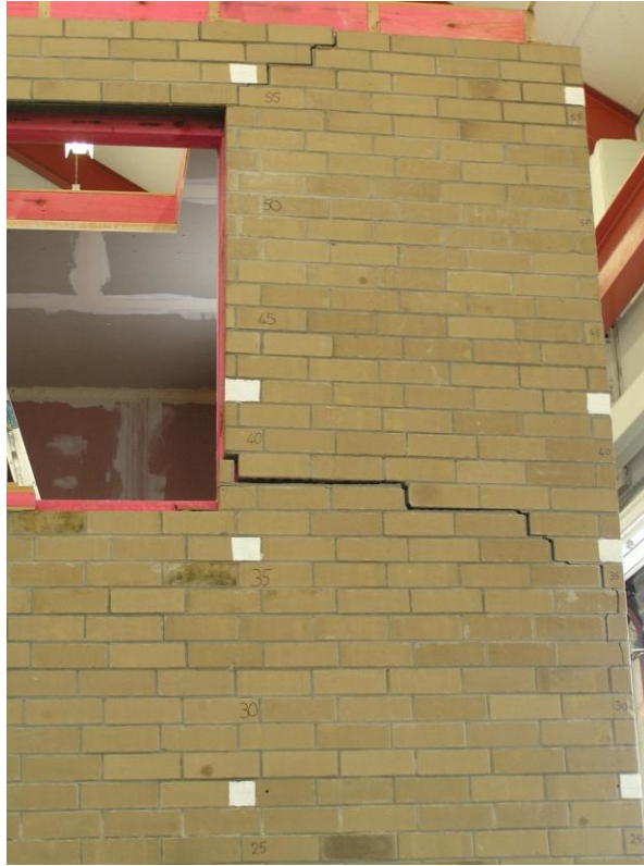
Figure 83. Cracking in Side 1 veneer at Panel C at peak push in Stage F
