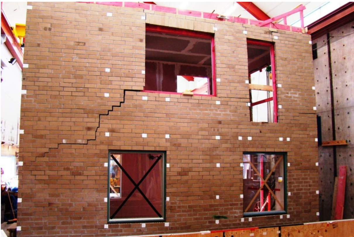
Figure 84. Cracking in Side 2 veneer at peak push in Stage F
