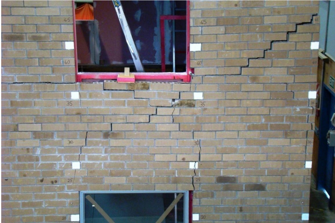
Figure 93. Cracking in Side 1 veneer at Corner 2 middle spandrel at peak pull in Stage G
