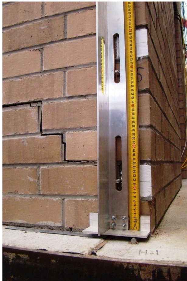
Figure 30. Measurement of veneer crack width by measuring height to scratch marks at eight locations up the height of the veneer
