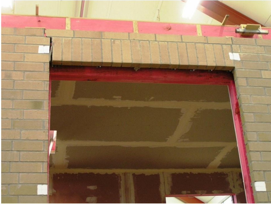
Figure 51. Lintel cracking above Side 2 Window C peak pull in Stage D
