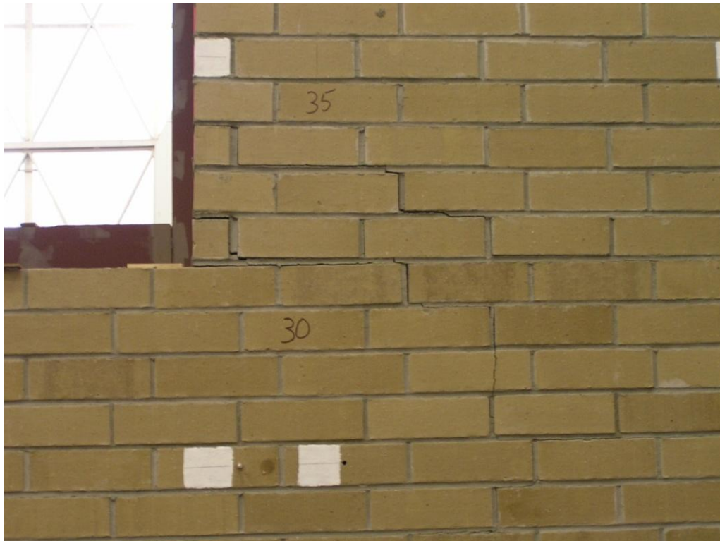
Figure 61. Cracking in Side 2 upper-storey veneer at Panel H at peak pull in Stage D
