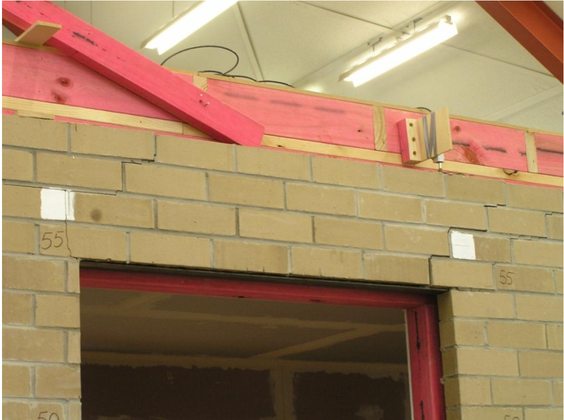
Figure 73. Residual cracking in Side 1 veneer above a top window at zero load after Stage E cycling
