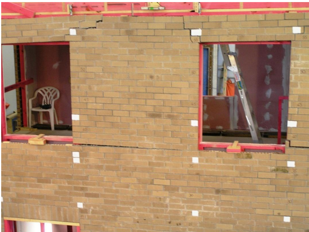
Figure 76. Cracking in Side 1 veneer at Panel B at peak push in Stage F
