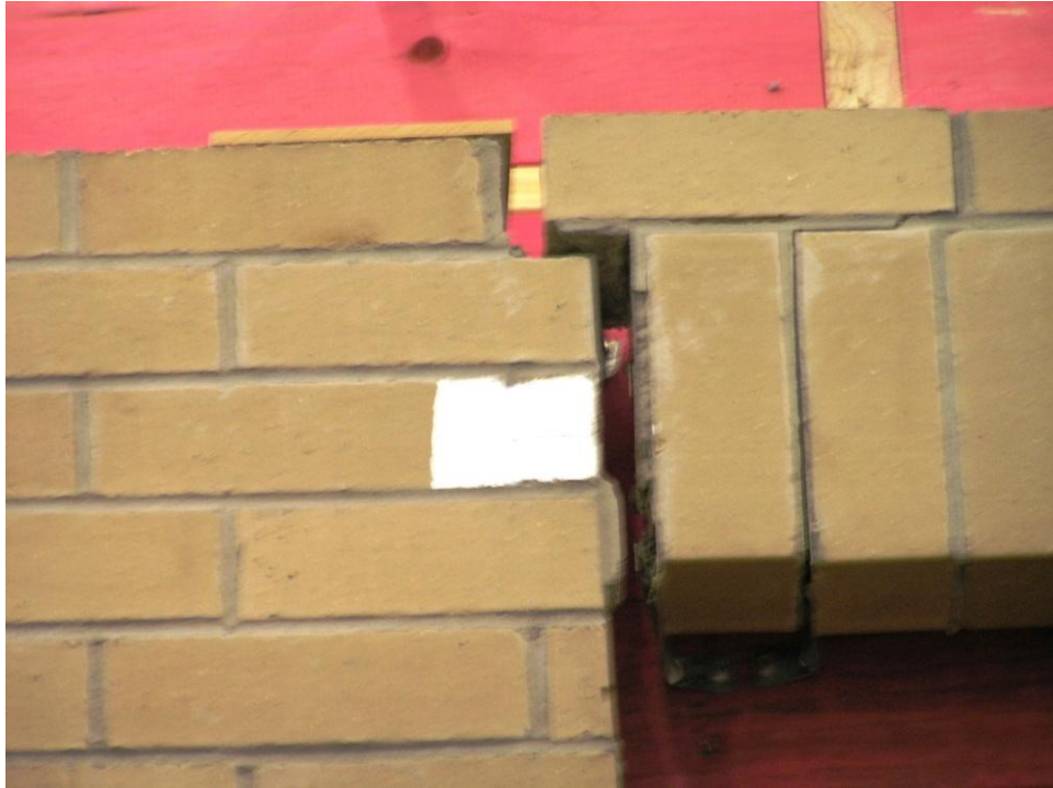
Figure 53. Lintel cracking above Side 1 Window S2C at peak pull in Stage F
