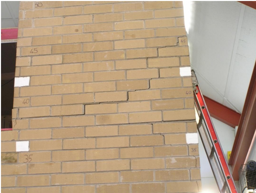
Figure 87. Cracking in Side 2 upper-storey veneer at Panel H at peak push in Stage F
