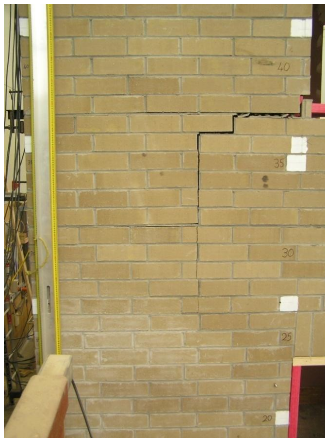
Figure 66. Cracking in Side 1 veneer at Panel A at peak pull in Stage E
