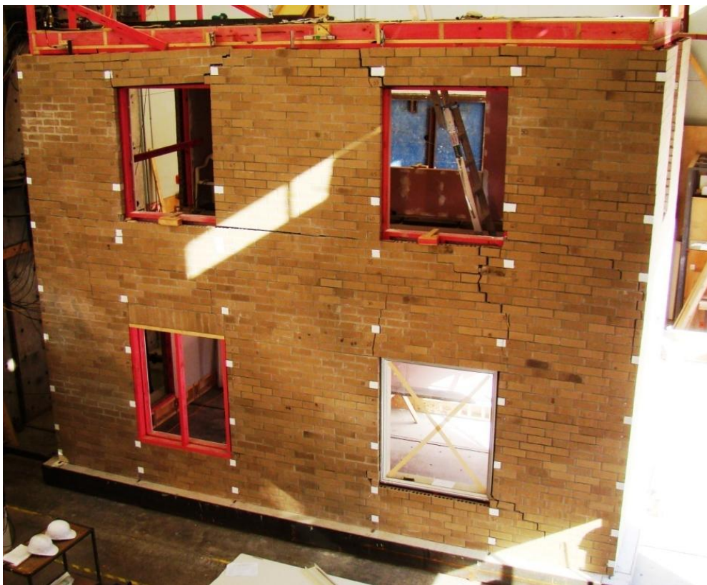
Figure 90. Cracking in Side 1 veneer at peak push in Stage G
