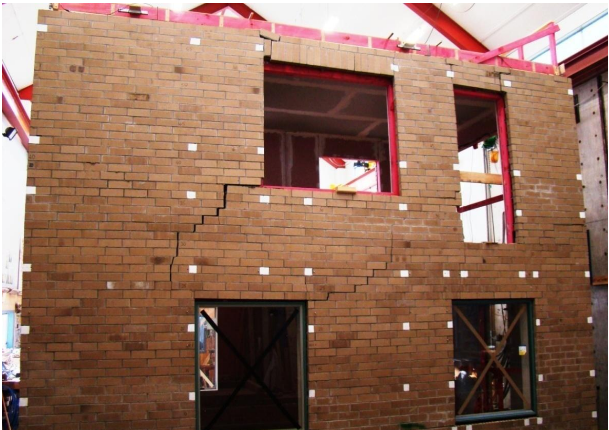
Figure 96. Cracking in Side 2 veneer at peak push in Stage G
