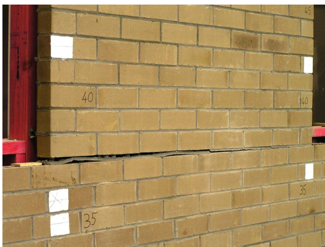
Figure 56. Cracking in Side 1 upper-storey veneer at Panel B at peak push in Stage D
