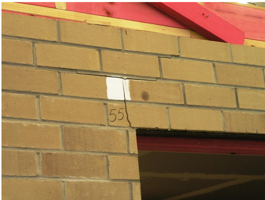
Figure 48. Lintel cracking above Side 1 Window S1D at peak push in Stage D
