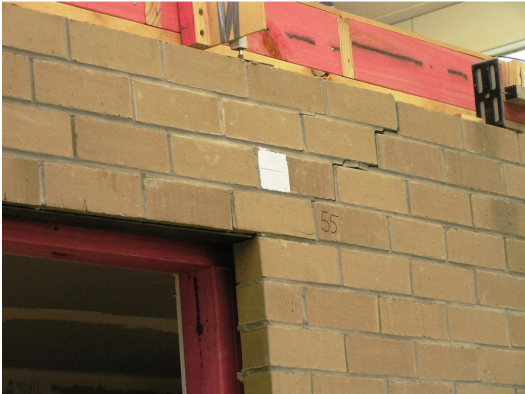
Figure 49. Lintel cracking above Side 1 Window S1C at peak push in Stage D
