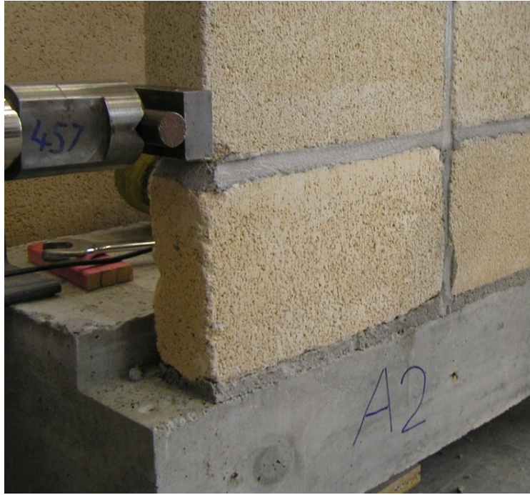
Figure 104. Concrete beam used as a foundation to fix bricks and application of shear load
