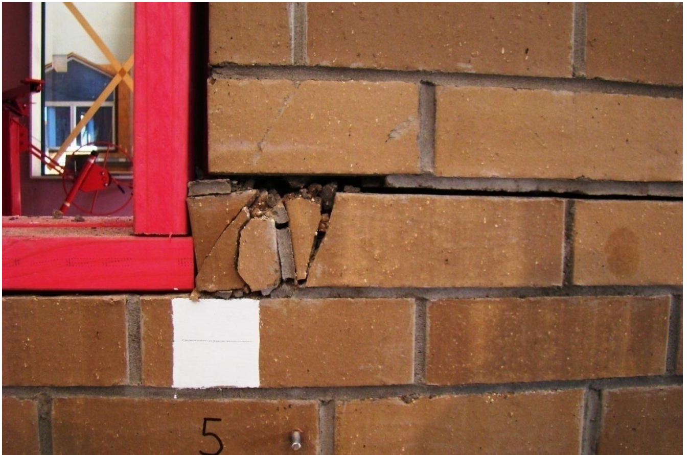
Figure 94. Brick crushing in Side 1 lower-storey veneer at Window S1B in Stage G
