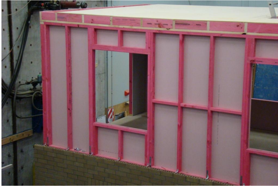
Figure 2. Laying brickwork against the LTF during construction
