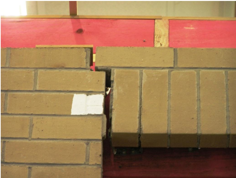
Figure 52. Lintel cracking above Side 2 Window S2C at peak pull in Stage E
