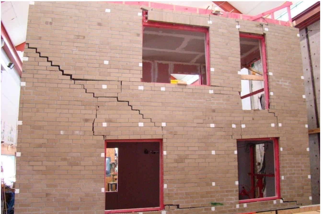
Figure 102. Cracking in Side 2 veneer at peak pull in Stage I
