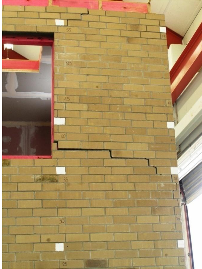
Figure 79. Cracking in Side 1 veneer at Corner 2 top window at peak push in Stage F
