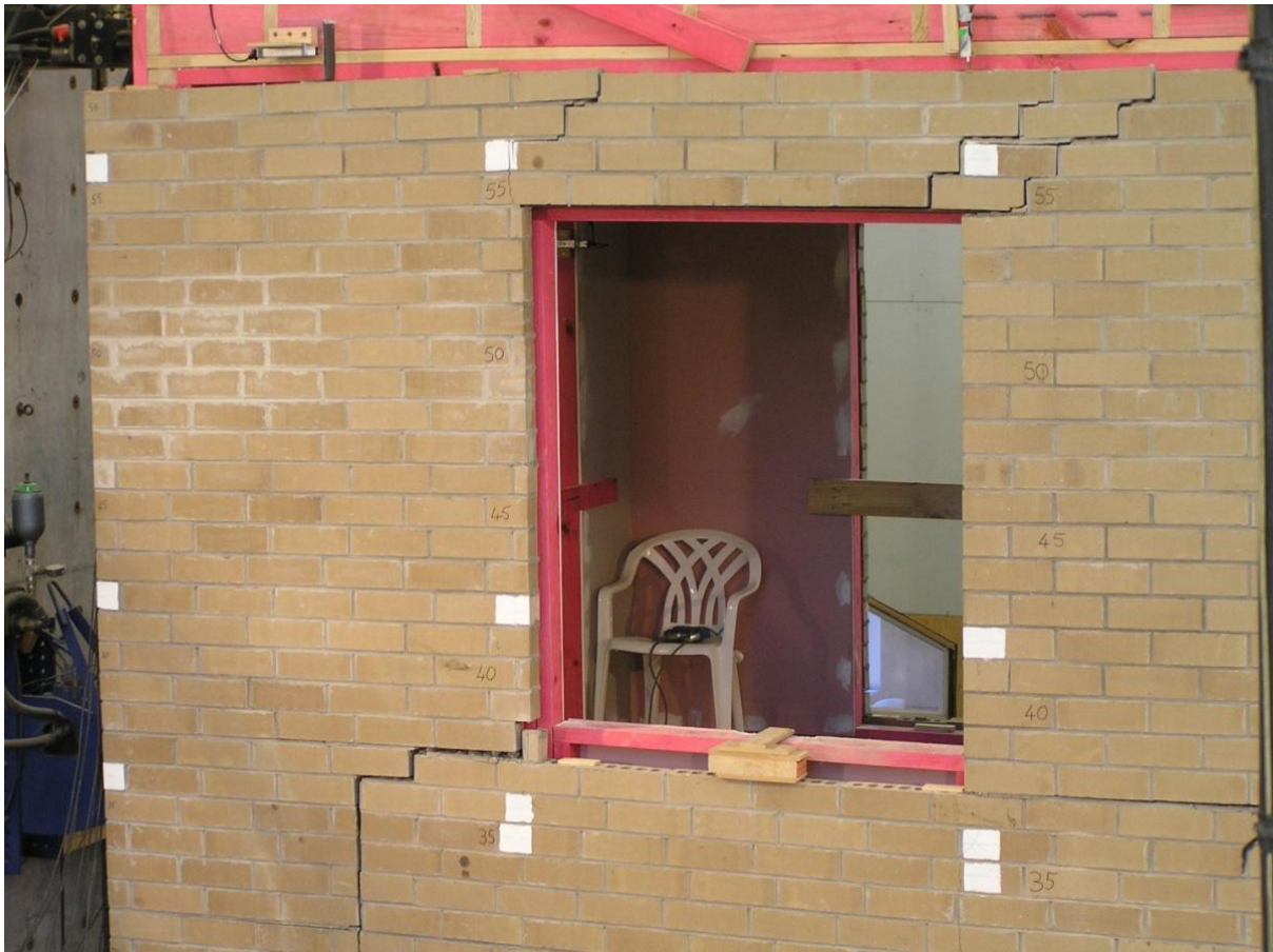
Figure 81. Cracking in Side 1 veneer at Corner 1 at peak pull in Stage F
