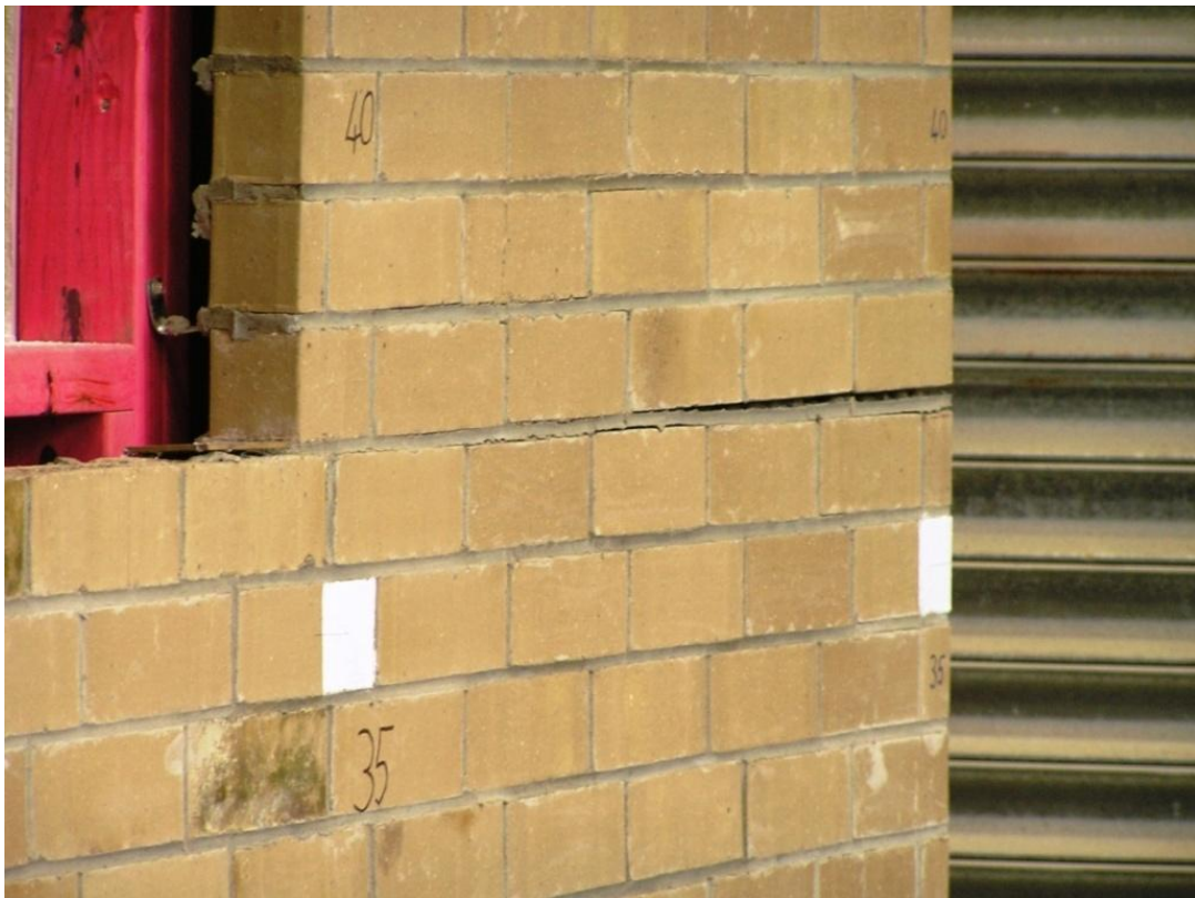
Figure 60. Cracking in Side 1 upper-storey veneer at Corner 2 at peak pull in Stage D
