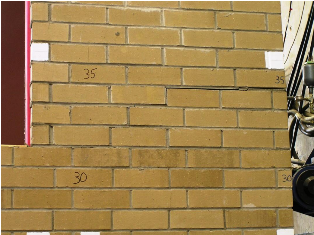
Figure 69. Cracking in Side 2 upper-storey veneer at Panel H at peak push in Stage E
