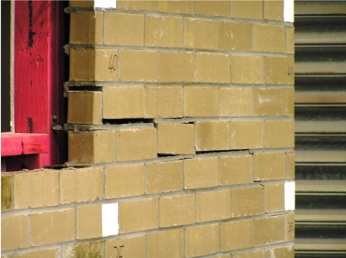
Figure 59. Cracking in Side 1 upper-storey veneer at Corner 2 at peak push in Stage D
