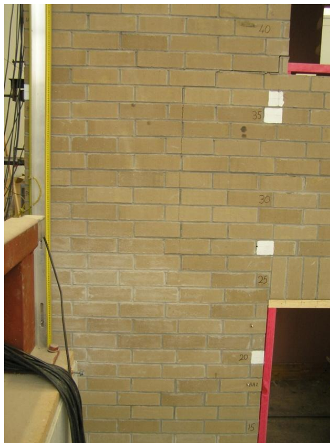
Figure 72. Residual cracking in Panel A Side 1 veneer at zero load after Stage E cycling
