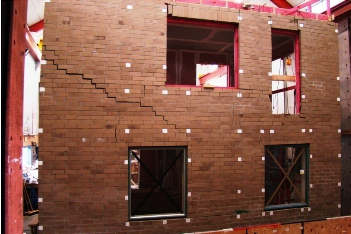
Figure 97. Cracking in Side 2 veneer at peak pull in Stage G
