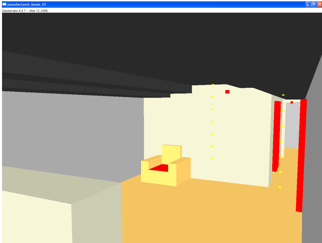
Figure 7. Smokeview representation of the modelled living room with armchair (the vent is located on the seat cushion of the armchair)
