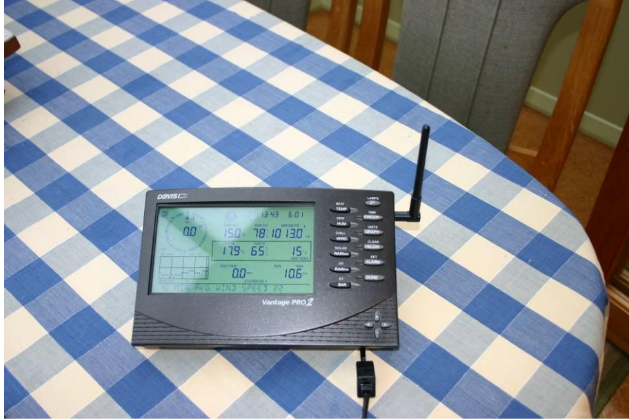
Figure 15. Console receiving data from the integrated sensor suite of the weather station. The data logger is located at the back of the console.
