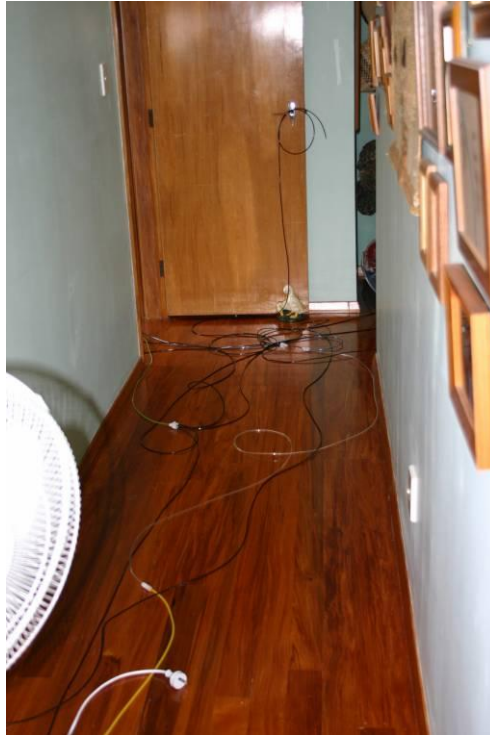
Figure 18. Pictures of part of the network of polyurethane tubes needed to inject tracer gases and draw air samples from different zones of the building.
