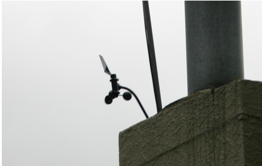
Figure 14. Anemometer mounted on the roof of one of the houses monitored.
