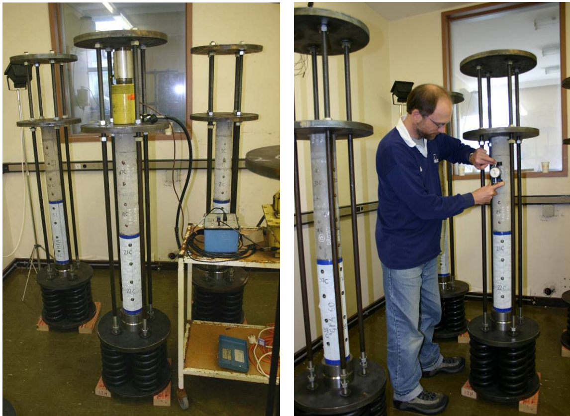
Figure 15: Creep testing rigs – load being applied with hydraulic jack (left) and induced strain being measured (right) with a Demec gauge (right)
