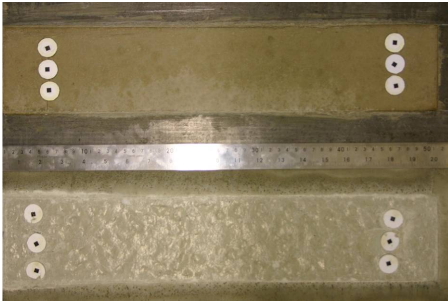
Figure 9: Example of the digital images captured for early age shrinkage analysis, showing the reference targets installed in the beam specimens
