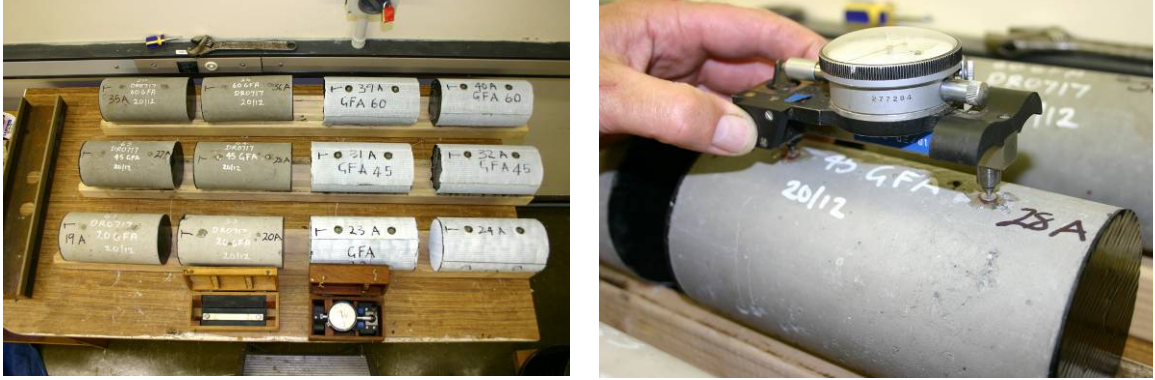
Figure 16: Unloaded ‘dummy’ cylinders, kept and measured to compensate for any deformation due to sources other than load
