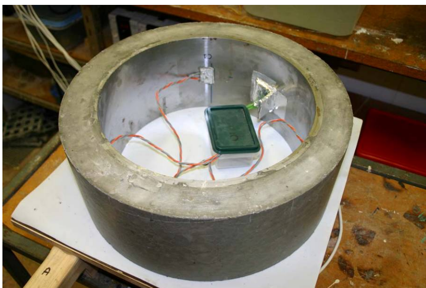
Figure 4: 20 GFA ring specimen after stripping
