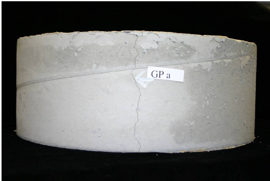
Figure 6: Control concrete restrained ring specimen, showing full wall thickness longitudinal crack
