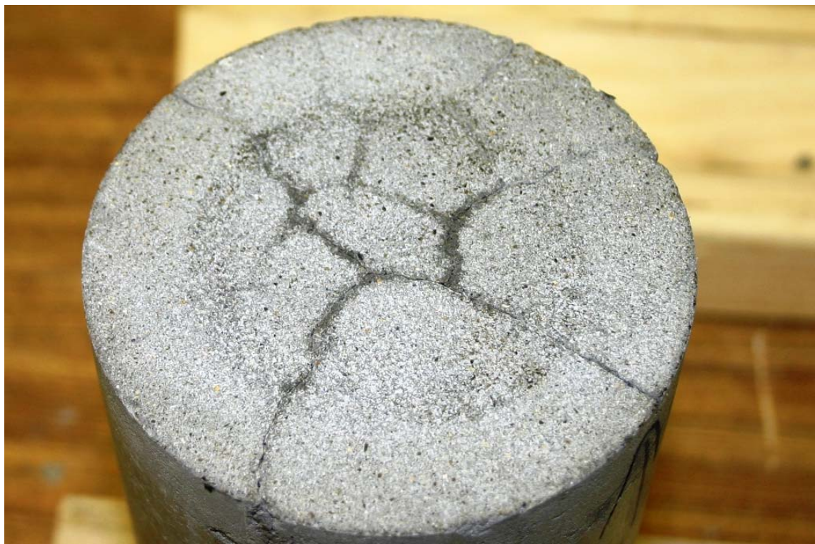
Figure 21: Examples of cracking developed in a 60 GFA dummy cylinder subjected to 'exposed' conditioning and storage
