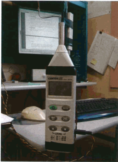
Figure 8. Sound level meter mounted to the post of the assembly array.
