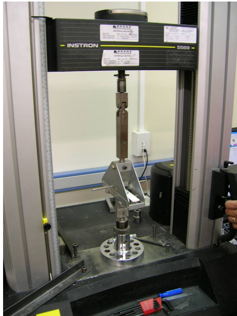
Figure 9. Flexural property testing.
