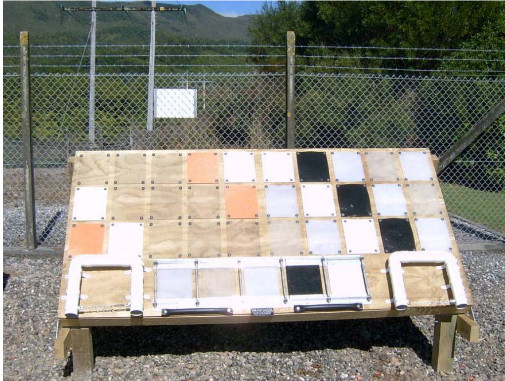
Figure 8. BRANZ exposure rack configuration (the composite materials are the white and pink/orange sheets on the left hand side of the exposure rack).
