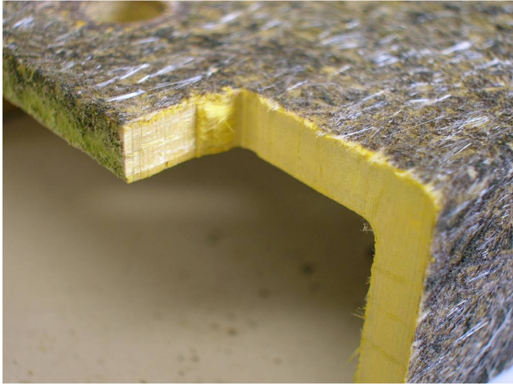
Figure 13. Exposed glass reinforcement at the surface of a pultruded FRP composite section after 22 years of exposure.
