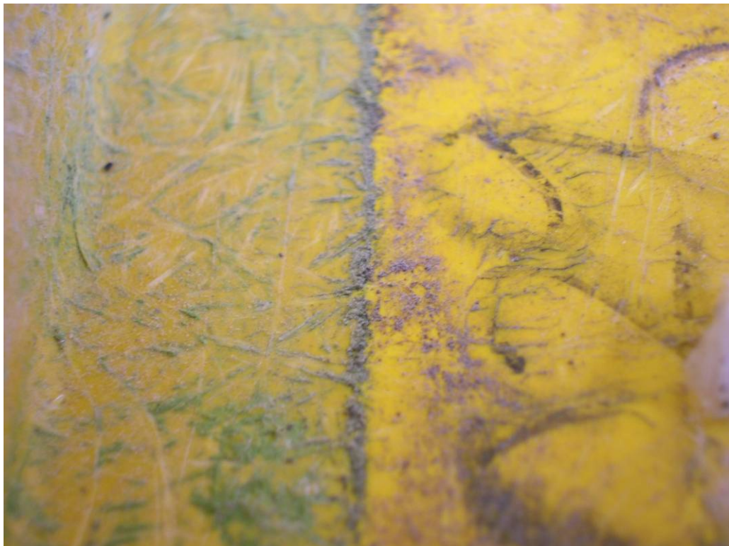
Figure 14. Evidence of exposure of the reinforcement on the sheltered area on the reverse of the pultruded sample (on the left of the photo) compared to the unexposed area on the right of the sample.
