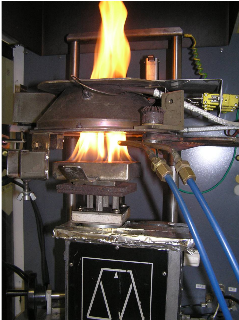
Figure 29. Cone calorimeter testing.
