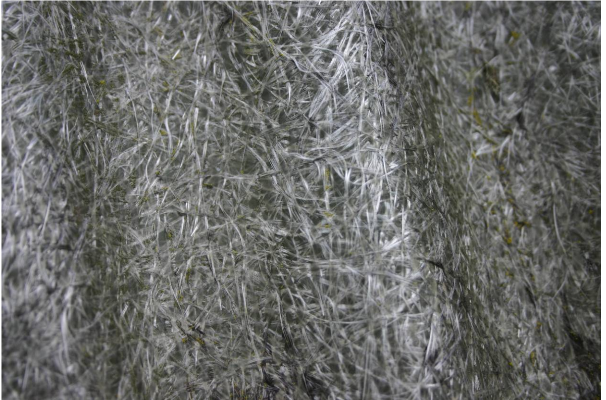
Figure 12. Exposed glass reinforcement at the surface of a polyester-based FRP composite following 19 years of exposure.
