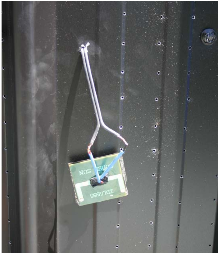
Figure 17. Installation of PV cell and surface of cladding.
