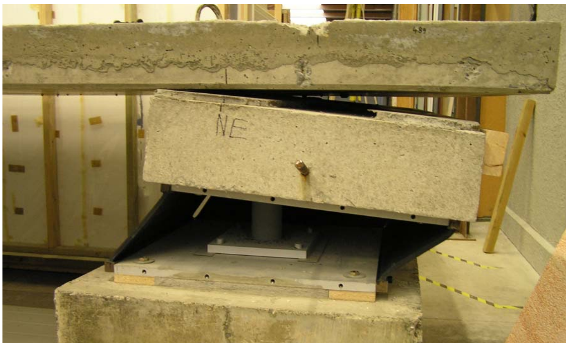
Figure 17. Static displacement to 140 mm with front ‘skirt’ removed.
