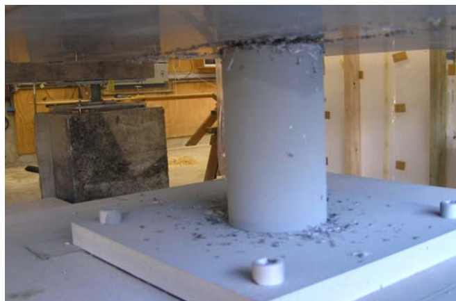
Figure 15. Wear on the Teflon pads.
