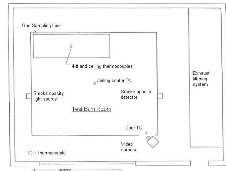
**Figure 49: TB 129 experimental set-up. Extracted from (Nurbakhsh & McCormack 1998).**
