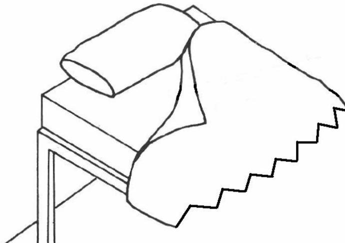
**Figure 40: Bedding assembly configuration for fire testing. Adapted from (Benisek, Phillips & Paul 1985).**
