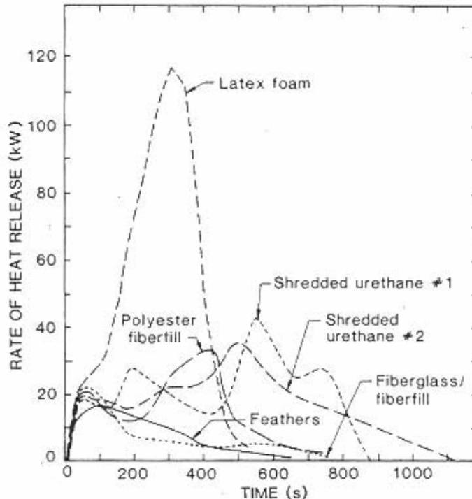
**Figure 52: HRR curves for various pillows. Extracted from (Babrauskas 1985).**
