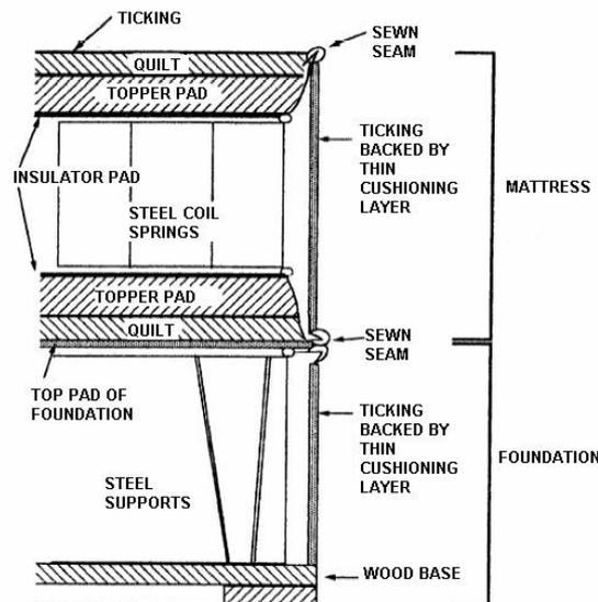
**Figure 50: Schematic of the cross-sectional view of the mattress and foundation structure. Extracted from (Ohlemiller 2003; Ohlemiller & Gann 2002, 2003; Ohlemiller, et al. 2000).**
