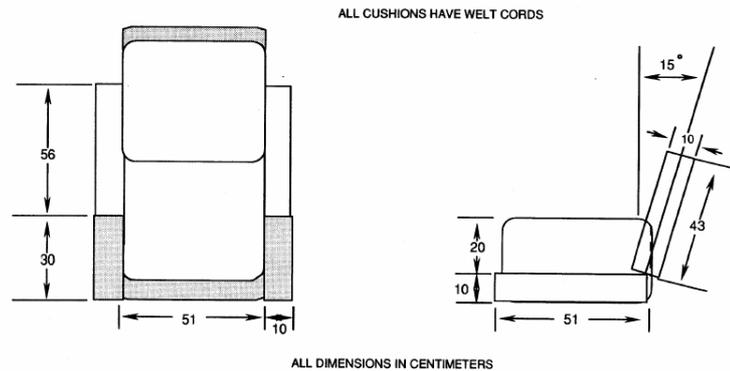
**Figure 63: Mock-up configuration. Extracted from (Ohlemiller & Shields 1995).**
