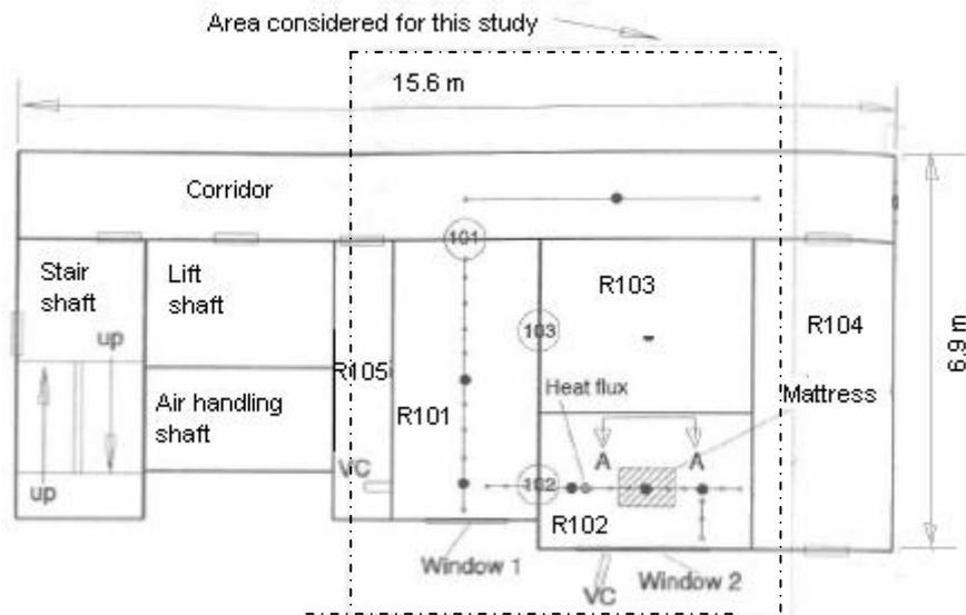
**Figure 47: Multi-room arrangement used for mattress fire testing by Luo and Beck. Extracted from (Luo & Beck 1996).**
