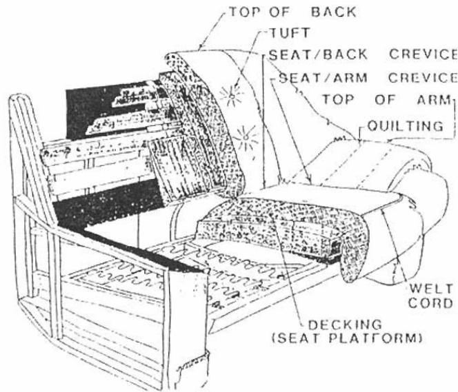
**Figure 58: Locations of ignition used for the testing of various chairs. Extracted from (McCormack, Damant & Hilado 1988).**
