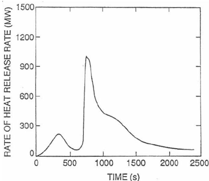
**Figure 62: The HRR curve for a 'nylon/fibreglass/TB 117' combination chair. Extracted from (Nurbakhsh 1991).**
