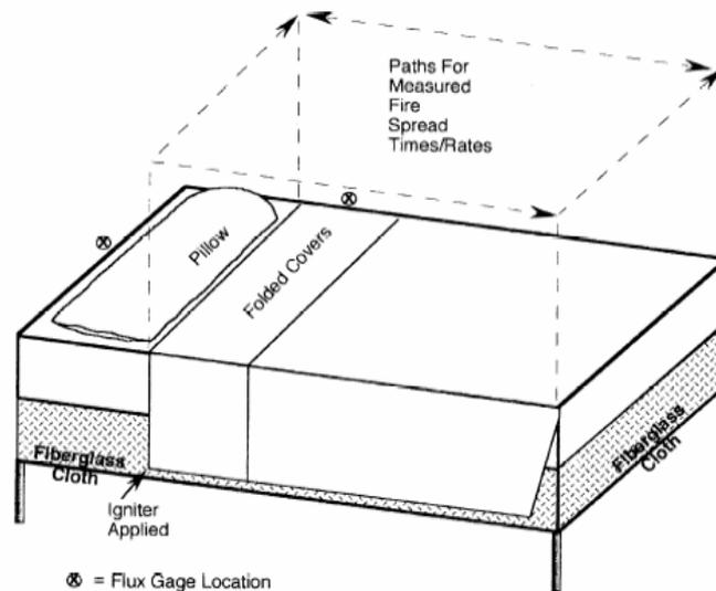
**Figure 51: Schematic of the set-up and igniter position for bedding tests on inert mattresses. Extracted from (Ohlemiller, et al. 2000).**
