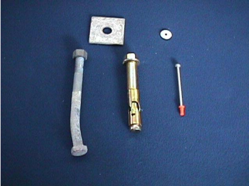
Photograph 1. Fasteners tested (L-R: M12 bolt, sleeve anchor, drive pin).
