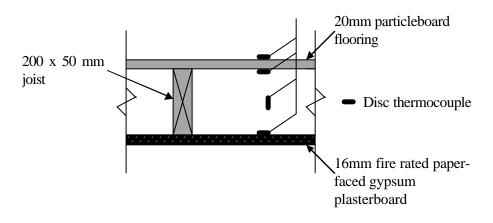
Figure 5: Room ceiling instrumentation layout
