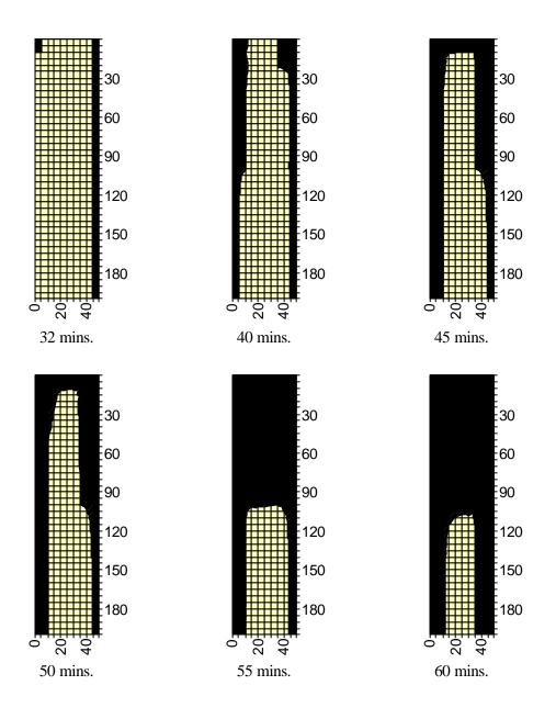
Figure 13: Dummy joist char diagrams
