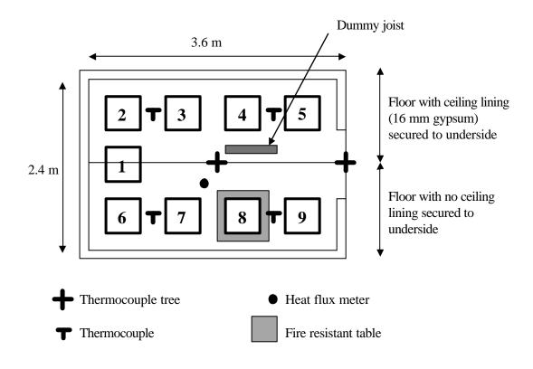
Figure 3: Diagrammatic layout of the room
