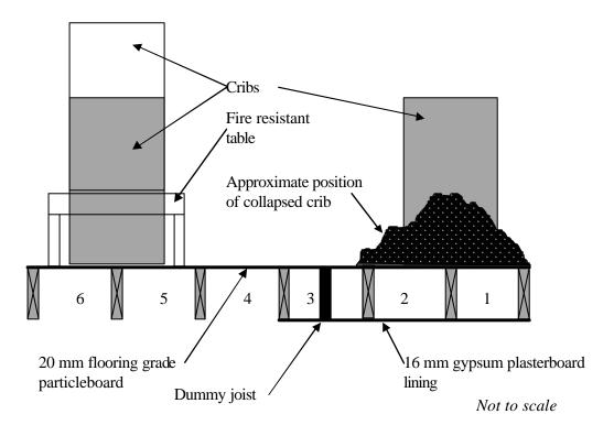
Figure 12: Diagrammatic section through room
