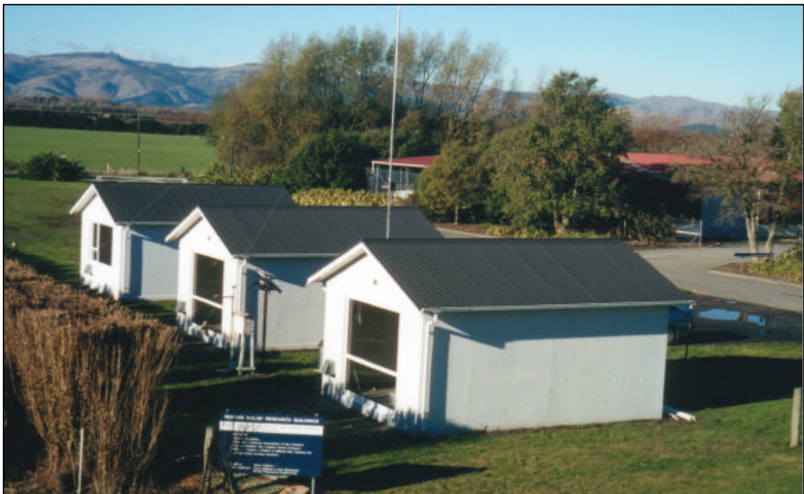
Figure 3. Side-by-side test buildings (before window overhangs were erected)
