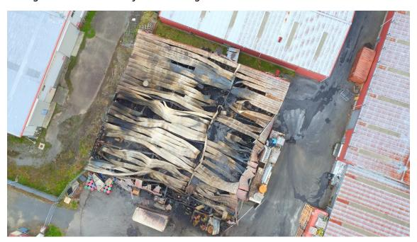
Figure 2. Aerial photo of the outcome of a fire in this type of building in New Zealand (Fire and Emergency New Zealand).
