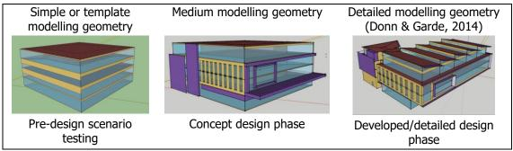
Figure 12. Illustration of energy model detail with design phase.
