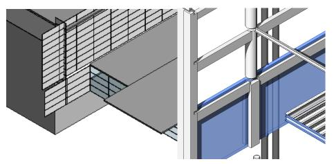
Figure 10. Example of BIM geometry required to obtain accurate material quantities.
