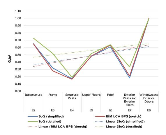
Figure 11. Example of post-calibration quality assurance results for one tested reference building.
