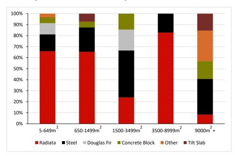
Figure 6. Wall infill framing found in surveyed office buildings.
