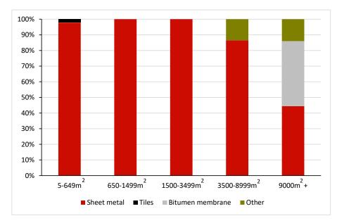
Figure 4. Roof claddings found in surveyed office buildings.
