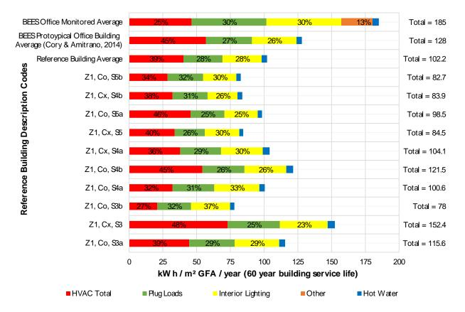
Figure 14. Comparison of module B6 operational energy.
