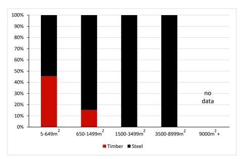
Figure 2. Roof structure found in surveyed office buildings.
