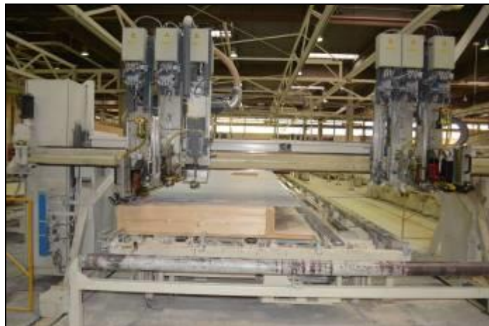
Figure 36: Automated equipment such as this automatic nailing bridge can be used to enhance the production line and supplement existing labour.
