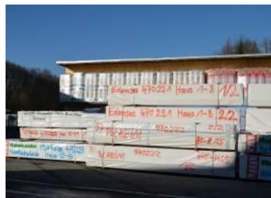
Figure 42: Wrapped and heat-sealed wall panels awaiting transportation in Austria.
