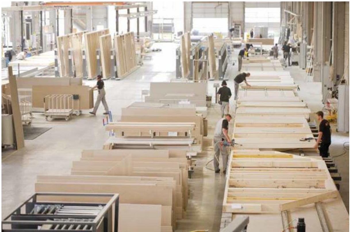
Figure 39: Fingerhaus factory production line for new housing in Hessen, Germany (Windsheif, 2013).
