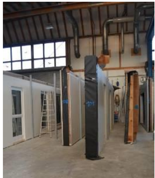
Figure 38: Closed timber-framed wall panels awaiting final touches at Huber and Sohn, Austria.
