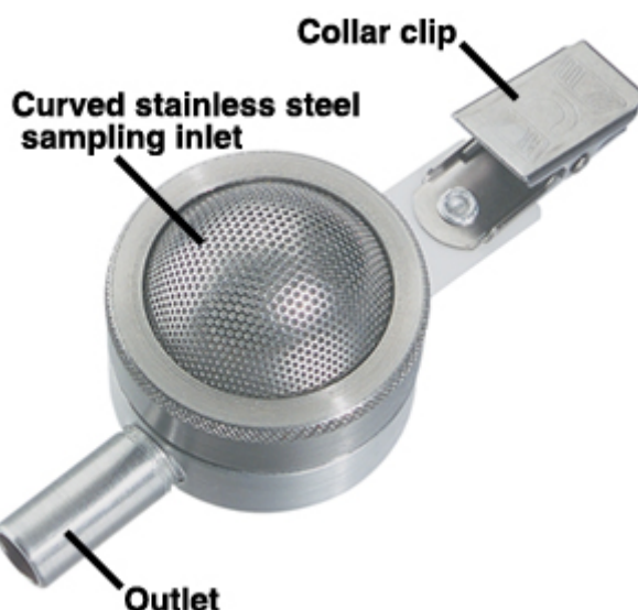
Figure 4: SKC button aerosol sampler (SKCinc.com)
