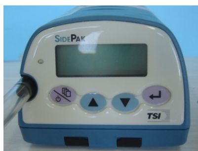
Figure 2: SidePak AM510 sampler
