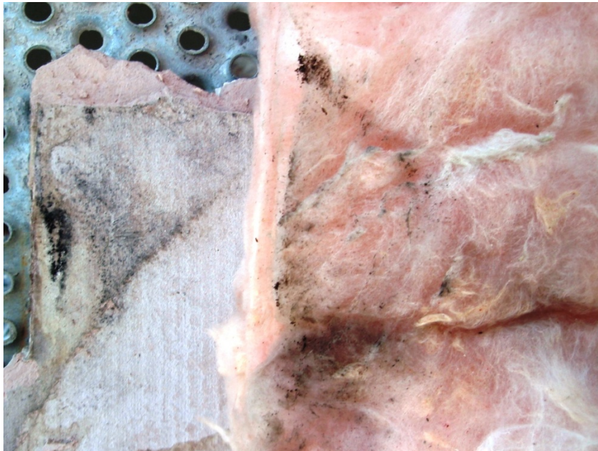
Figure 24: (Photo 24) Visible 'soot-like' biocontamination of fibre cement (left) and insulation batts (right) by toxigenic fungus Stachybotrys chartarum .
