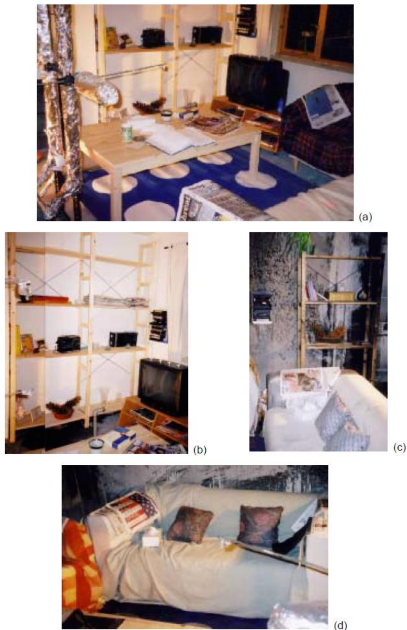
Figure 22: An example of the furnished lounge setup in the house fire test (Williams and Campbell, 2004)
