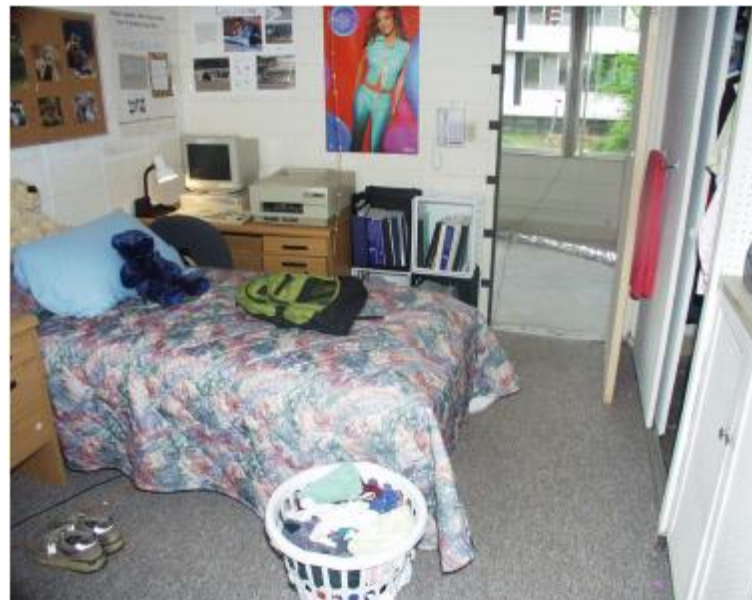
Figure 17: Example of the bed fuel package used in the sleeping room tests (Madrzykowski and Walton, 2010)
