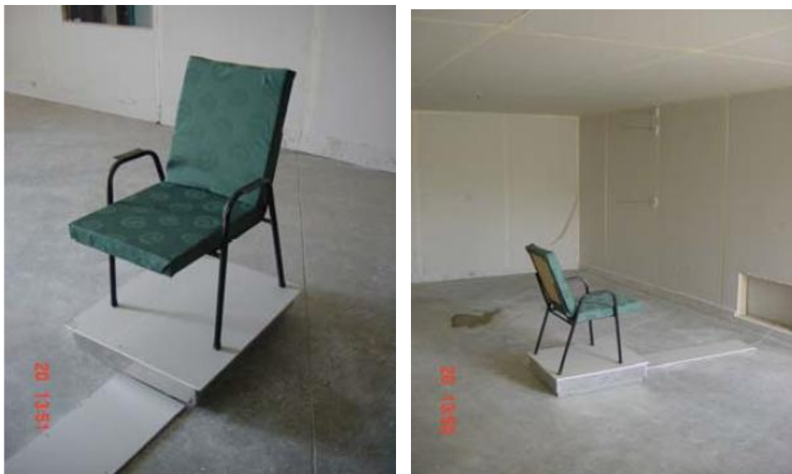
Figure 33: Chair used as the fuel package for the chair and two sprinkler head compartment tests (Bittern, 2004)
