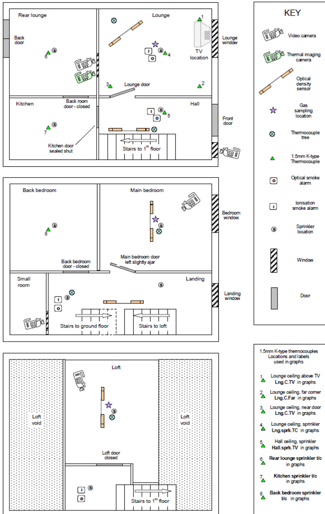
Figure 21: Schematic of the house and instrumentation used for fire testing (Williams and Campbell, 2004)
