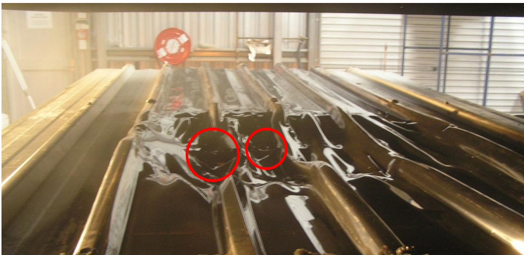
Figure 92: Openings formed in panel. (Test 16 at 21 min after ignition of burner.)
