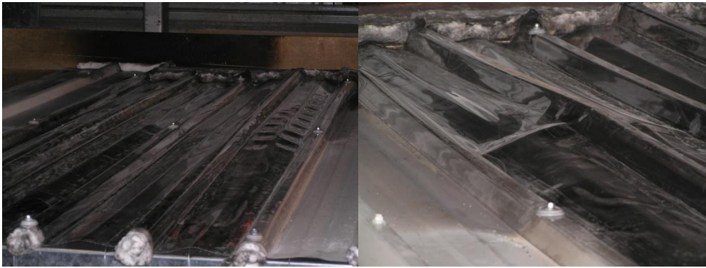
Figure 70: Slight sagging and wrinkling of panel. (Test 14 at 14 min from ignition of burner.)
