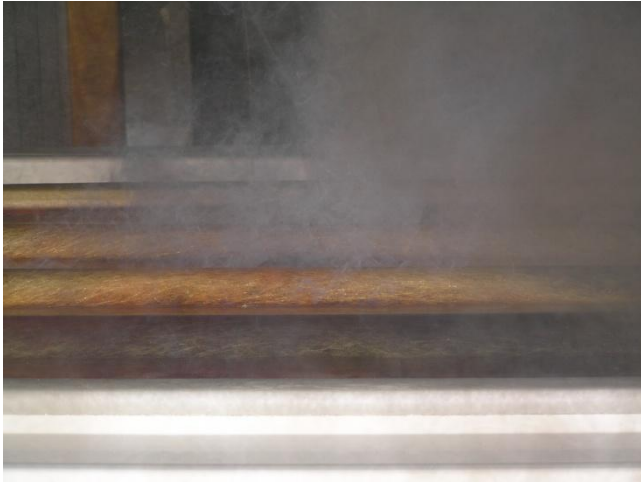
Figure 62: Topside of panel, showing smoke rising from surface. (Test 13 at 27 min from ignition of burner.)
