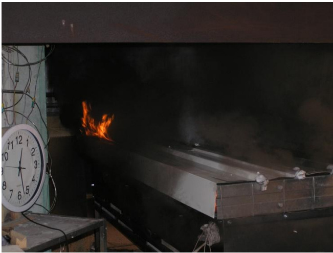
Figure 63: Heavy smoke and flames from burning panel. Burner is off. (Test 13 at 20 s after burner was switched off).
