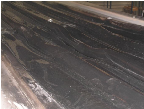
Figure 79: Panel further sagging. (Test 15 at 18.5 min from ignition of burner.)
