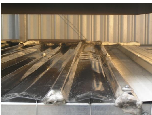
Figure 76: Deformation of the panel. (Test 15 at 13 min from ignition of burner.)
