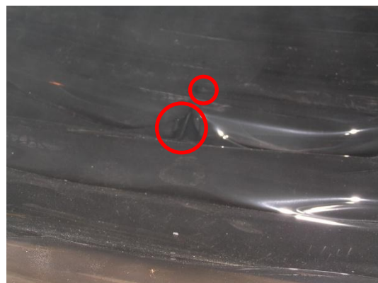
Figure 80: Opening forming. (Test 15 at 21 min from ignition of burner.)
