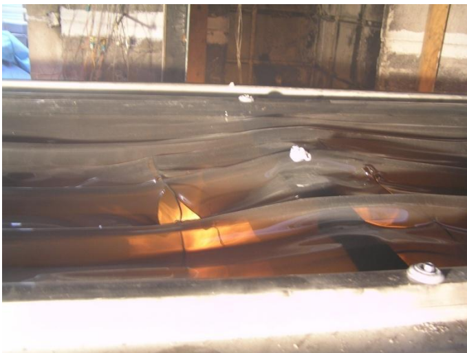
Figure 106: Flames seen around edges of baffles. (Test 19 at 21.5 min from ignition of burner.)
