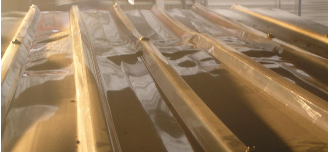
Figure 104: Deformation of panel. (Test 19 at 12 min from ignition of burner.)
