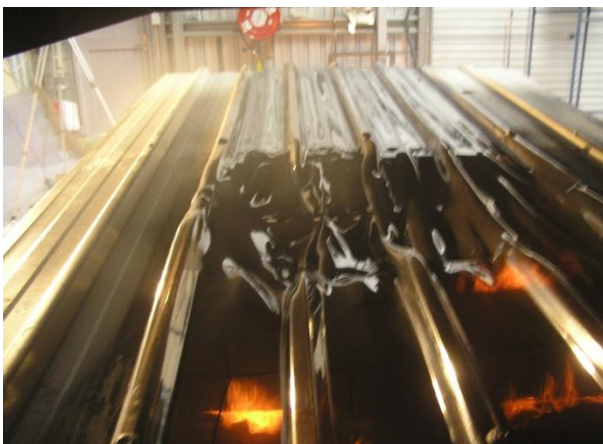
Figure 93: Observed burner flames around edges of panel. (Test 16 at 23 min after ignition of burner.)
