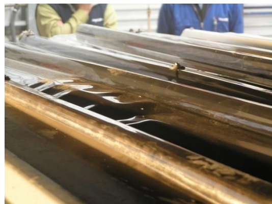
Figure 76: Deformation of the panel. (Test 15 at 13 min from ignition of burner.)
