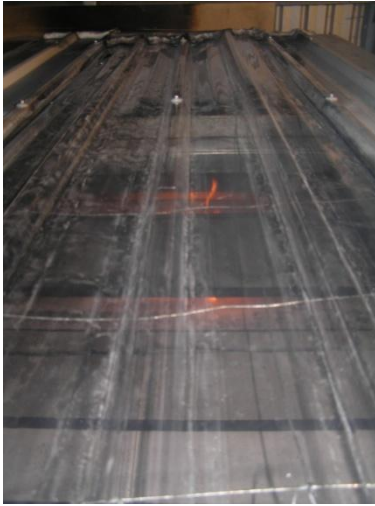
Figure 69: Small intermittent flames around the edges of the centre-most baffles, as observed through the transparent panel. (Test 14 at 5 min from ignition of burner.)
