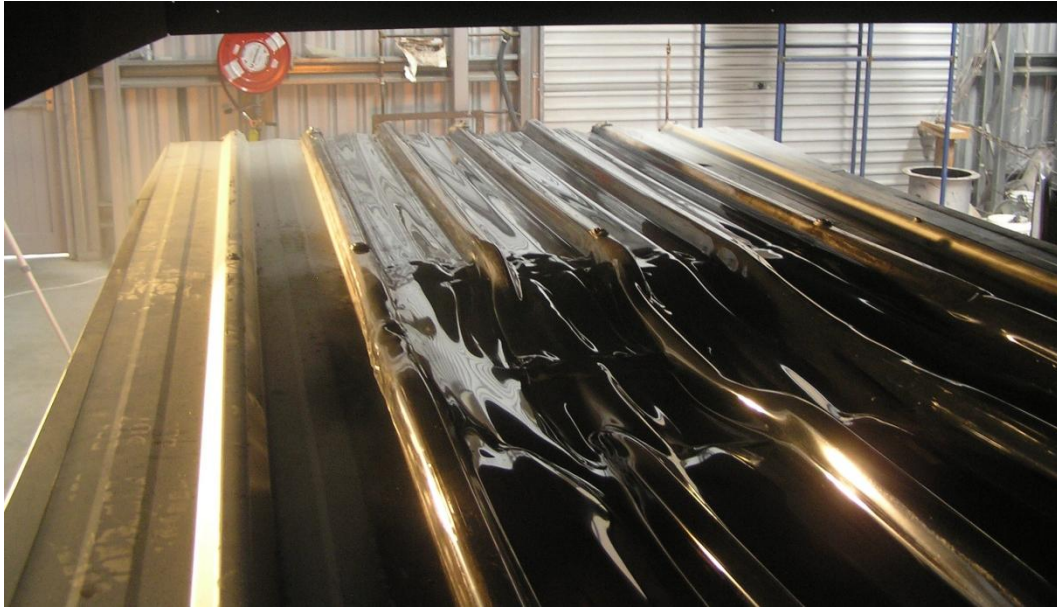
Figure 91: Further sagging of panel. (Test 16 at 20.5 min after ignition of burner.)
