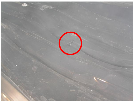
Figure 80: Opening forming. (Test 15 at 21 min from ignition of burner.)
