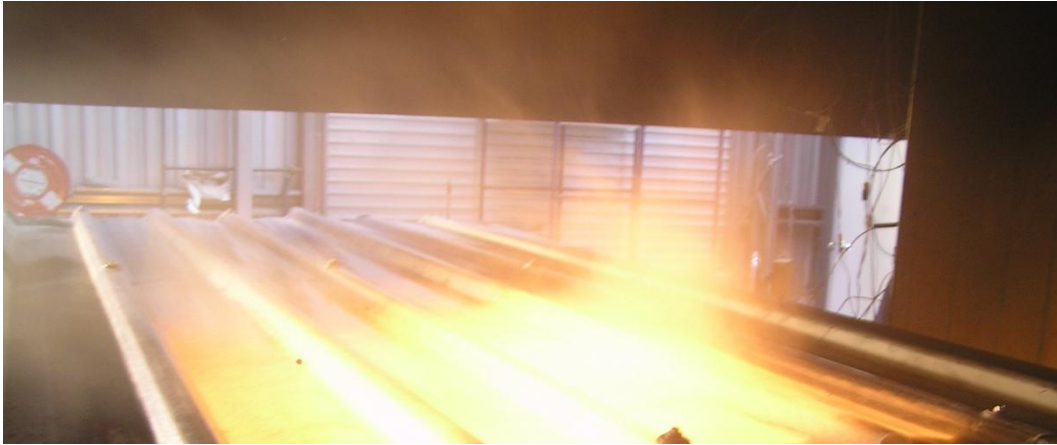
Figure 112: Flaming on underside of panel and smoke rising from topside of panel. (Test 20 at 105 s from ignition of burner.)
