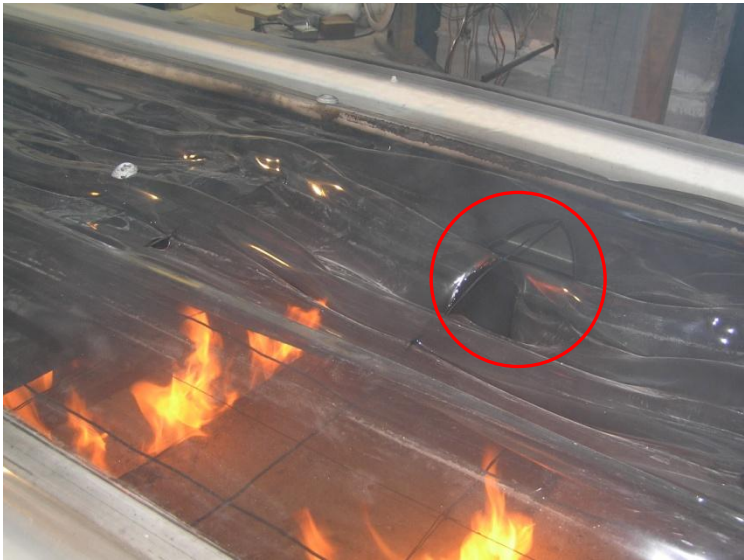
Figure 72: Openings (circled in red) formed in panel. (Test 14 after 18.25 min from burning ignition.)
