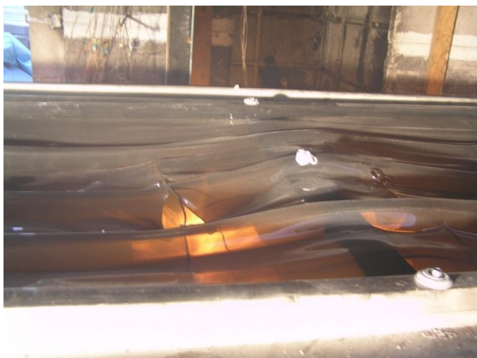
Figure 9: Flames seen around edges of baffles. (Test 19 at 21.5 min from ignition of burner.)
