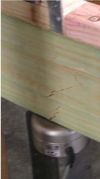
Figure 35. Test L2 – crack in joist
