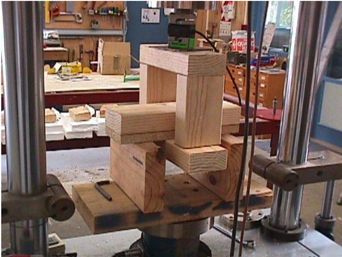
Figure 51. Test set-up used to measure bottom plate to timber joist tension strength
