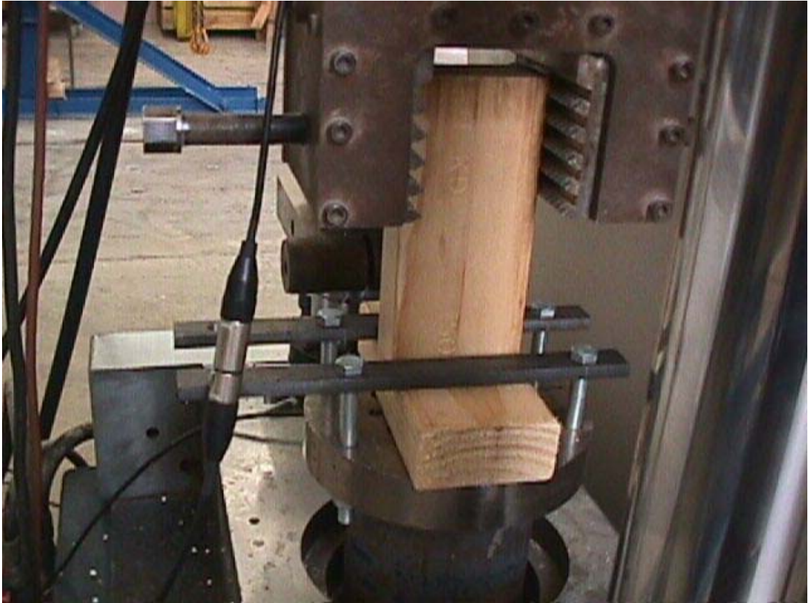
Figure 49. Test set-up used to measure stud/plate tension strength
