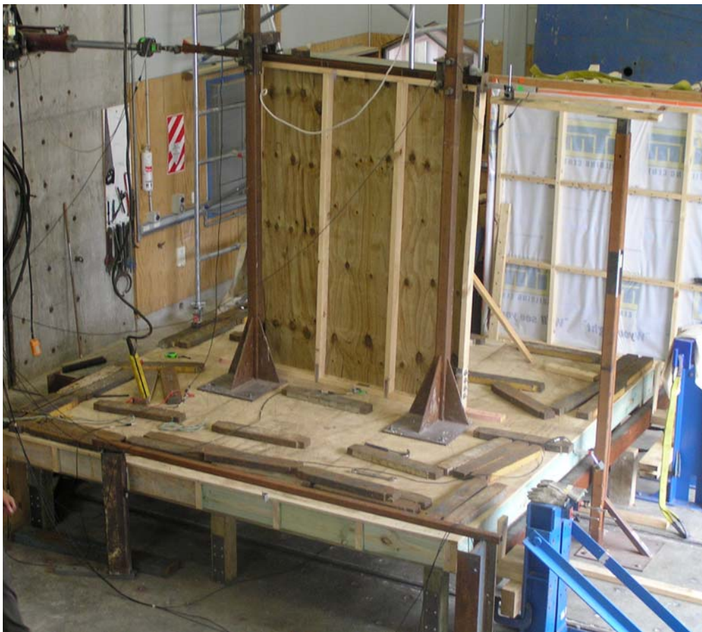
Figure 44. Test L4 – specimen at peak push load
