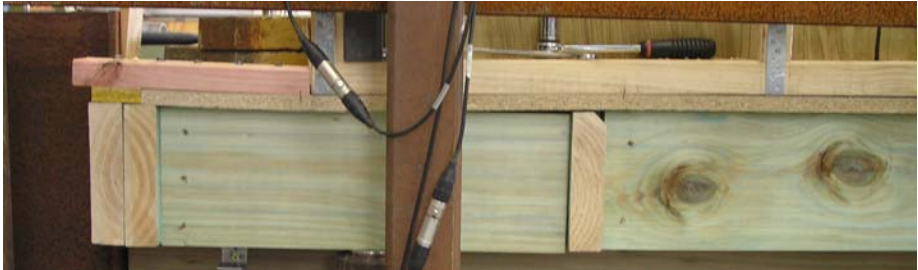
Figure 30. Test L1 – uplift at racking force of 8.42 kN pull at compression end of wall
