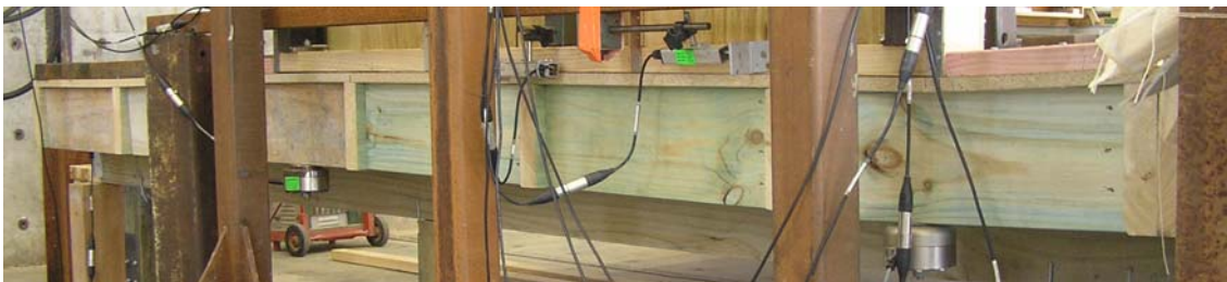
Figure 42. Deflections along the loaded side of Test L3
