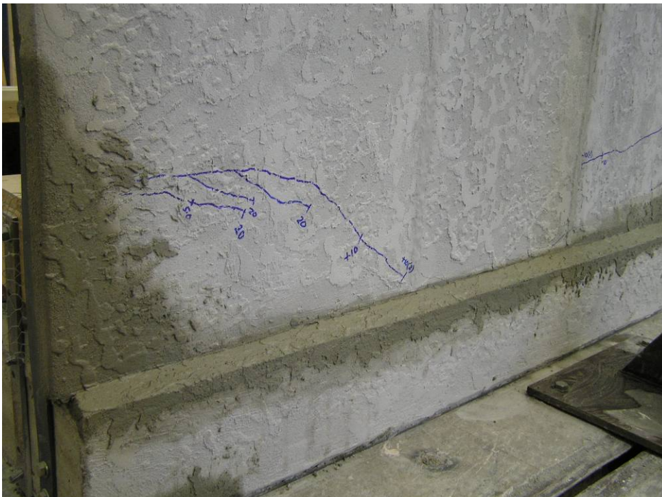
Figure 8: Repaired stucco wall at foundation junction and at the wall ends
