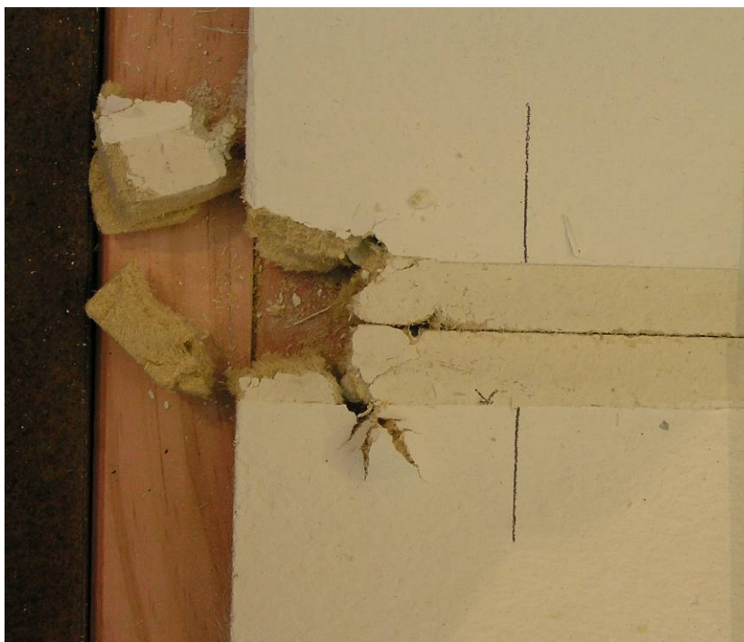
Figure 24: Breakout of the sheet corners
