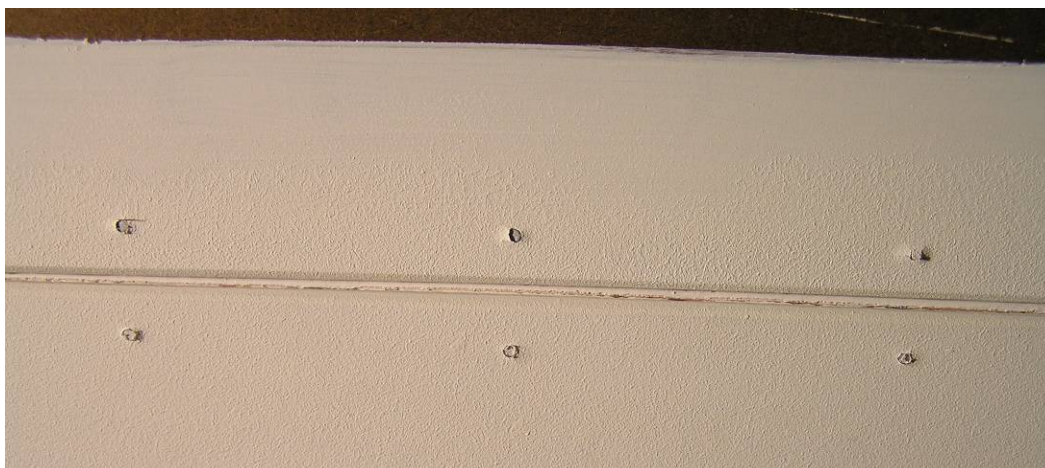
Figure 28: Panel pin heads becoming clearly visible during cycling to \pm 20 mm
