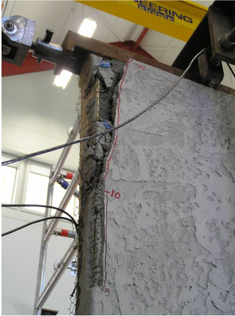
Figure 10: Damage at the top corners of the panel
