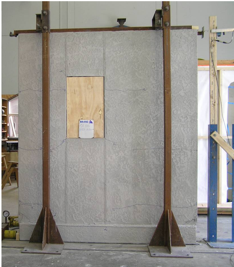
Figure 6: Crack patterns after cycling to \pm 10 mm (note cracks have been marked with a felt-tip pen)
