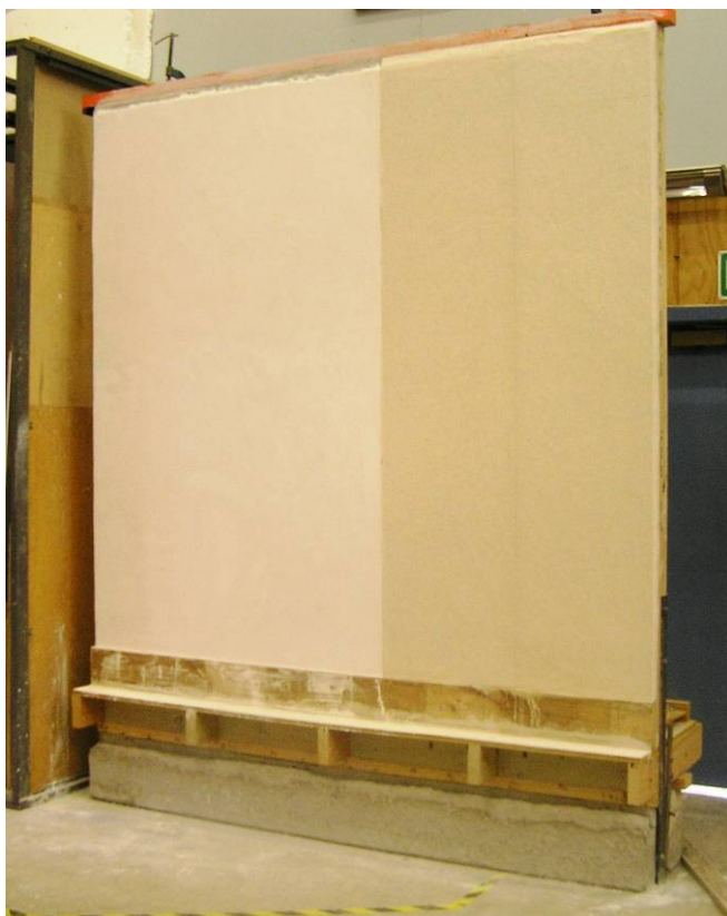
Figure 35: Completed lath and plaster wall with casting plaster top coat (left side) and wallpaper over second coat (right side)
