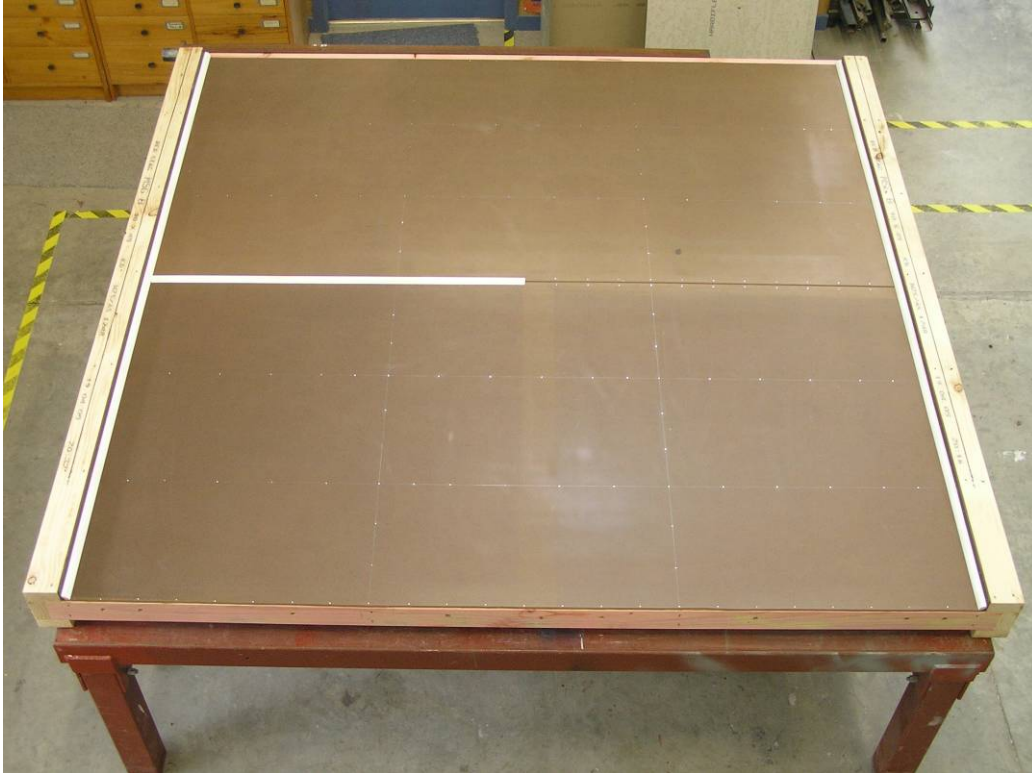
Figure 26: View of the hardboard test specimen before installation in the test rig
