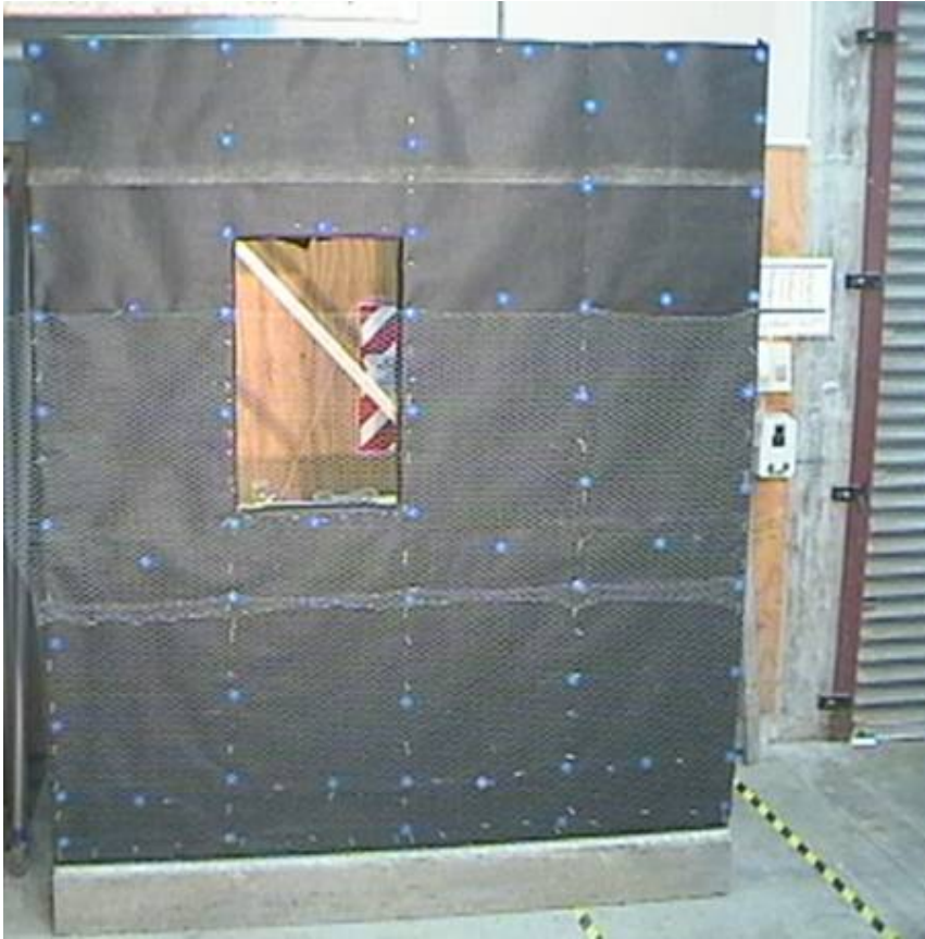
Figure 1: Building paper in place and chicken wire being added
