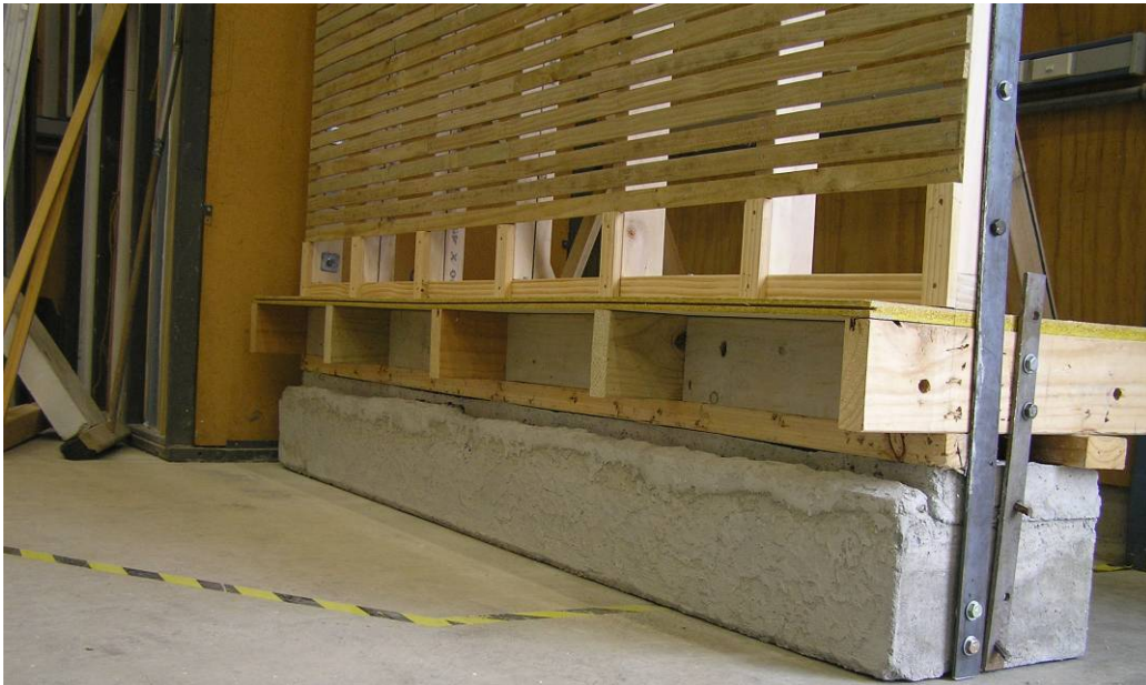
Figure 32: Timber framing for the lath and plaster wall
