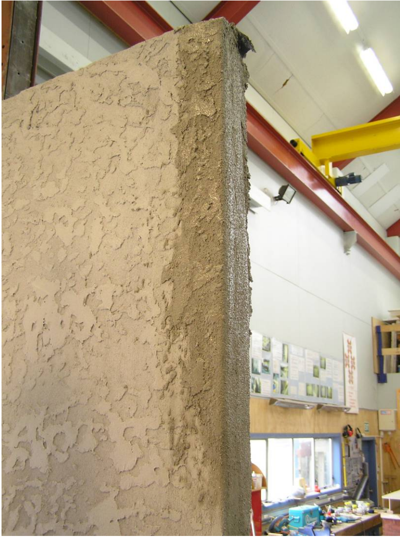
Figure 11: Top corners of the stucco wall after repair
