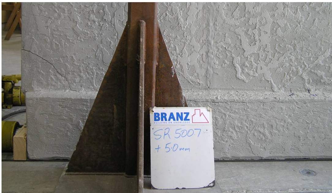
Figure 5: Cracks extending along the foundation junction during cycles to \pm 5 mm
