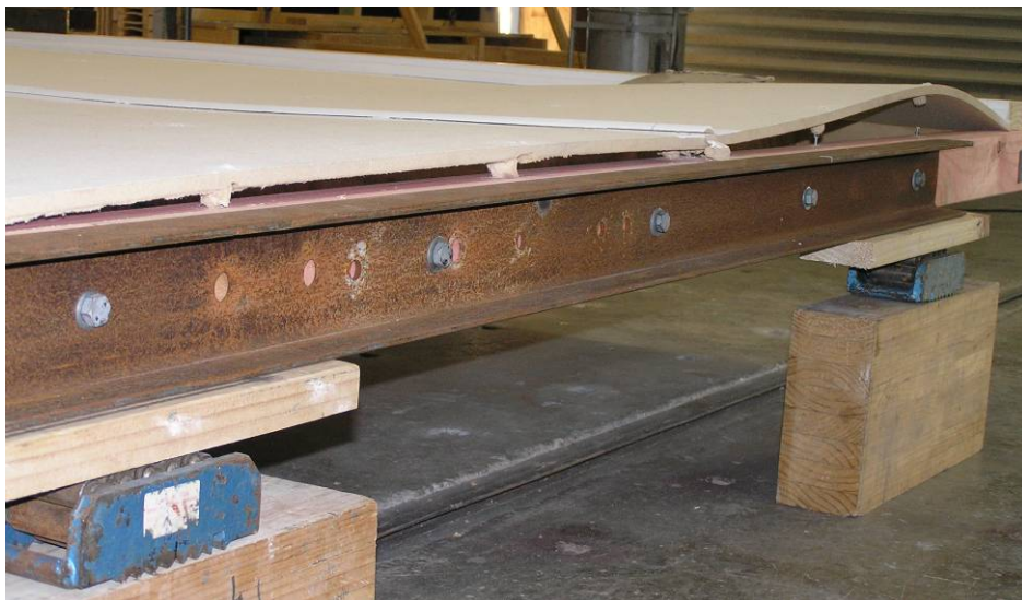
Figure 23: Buckling of the sheet edges at 40 mm displacement
