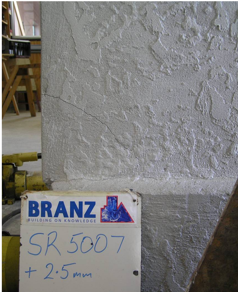
Figure 4: Fine crack at the bottom of the wall and at the junction with the concrete foundation
