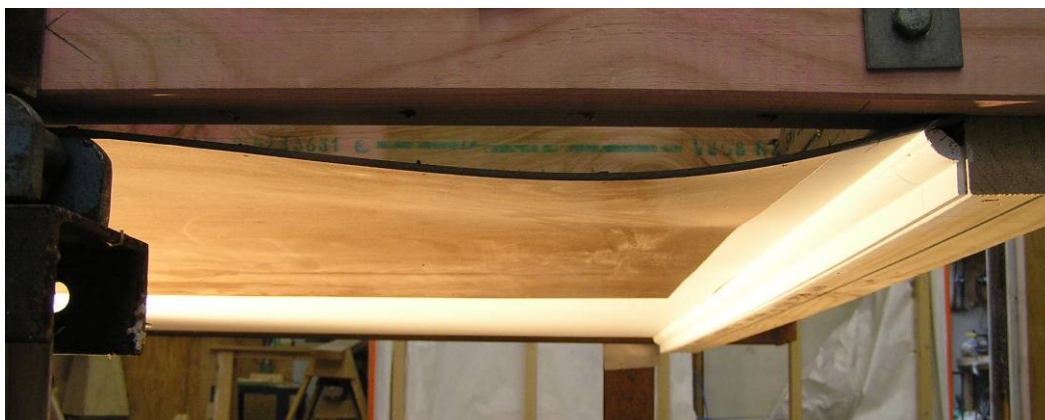
Figure 29: Hardboard detached from the framing during the \pm 40 mm cycle
