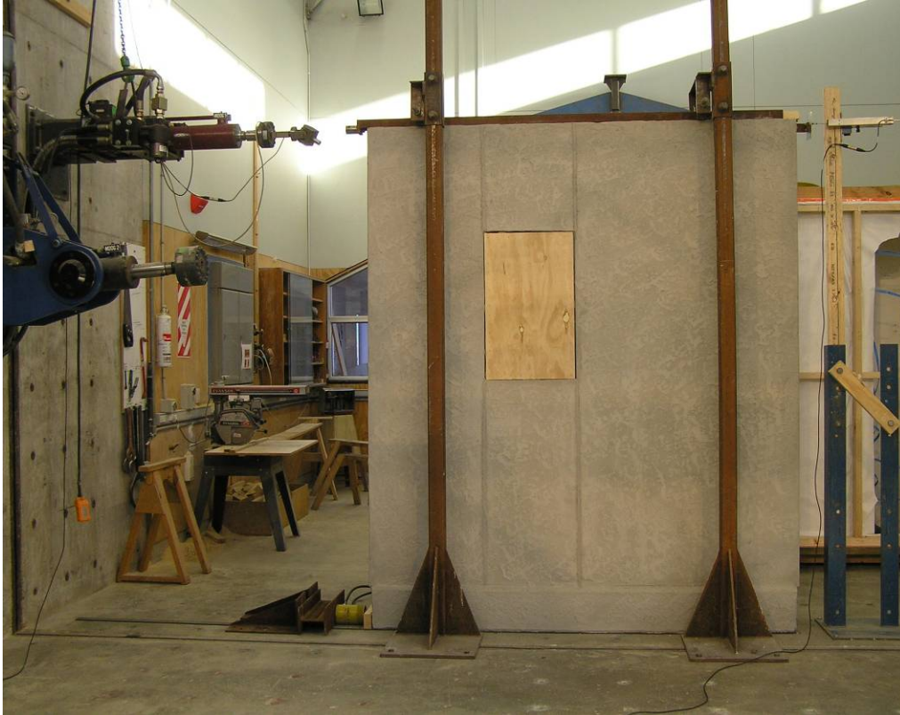
Figure 3: Stucco specimen ready for loading
