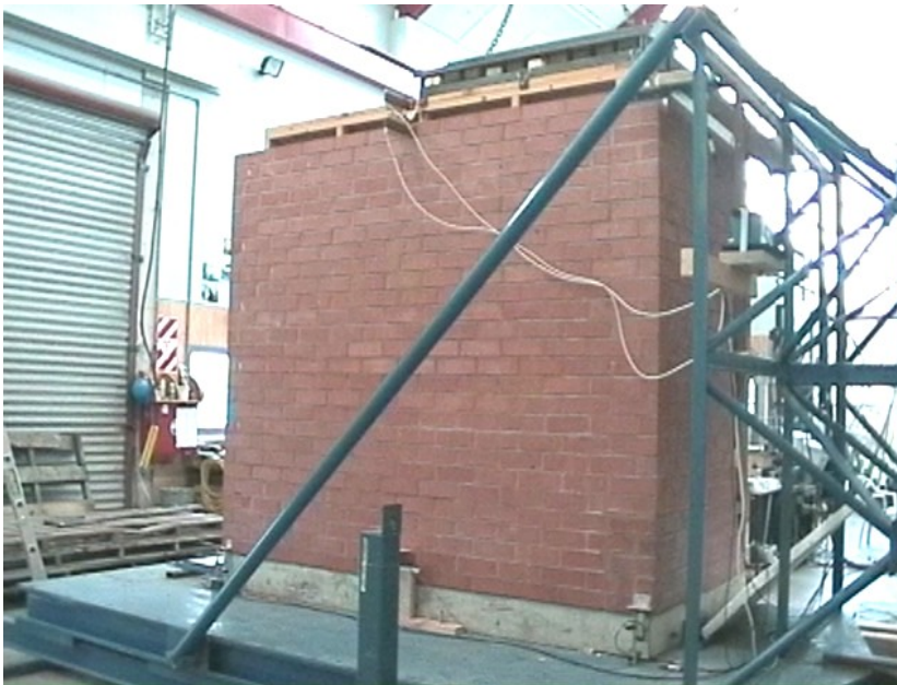
Figure 2: Veneer test specimen mounted on shake table
