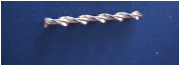
Figure 1: View of a proprietary tie (note that the ties used for tying the veneer were longer than shown)
