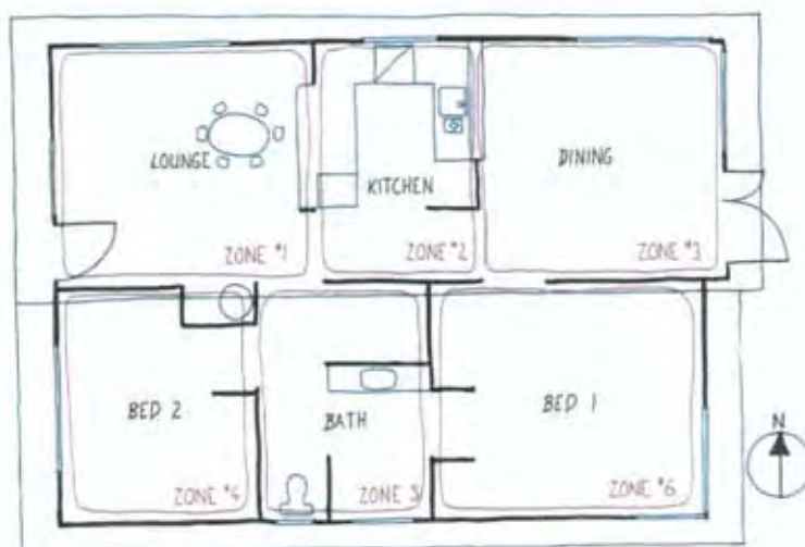
Figure 4: Schematic of the small house. The total floor area is 81 m 2 . The lounge, kitchen and dining rooms are the most important living spaces in terms of overheating. The house is modelled as having seven different temperature zones (including the roof space).
