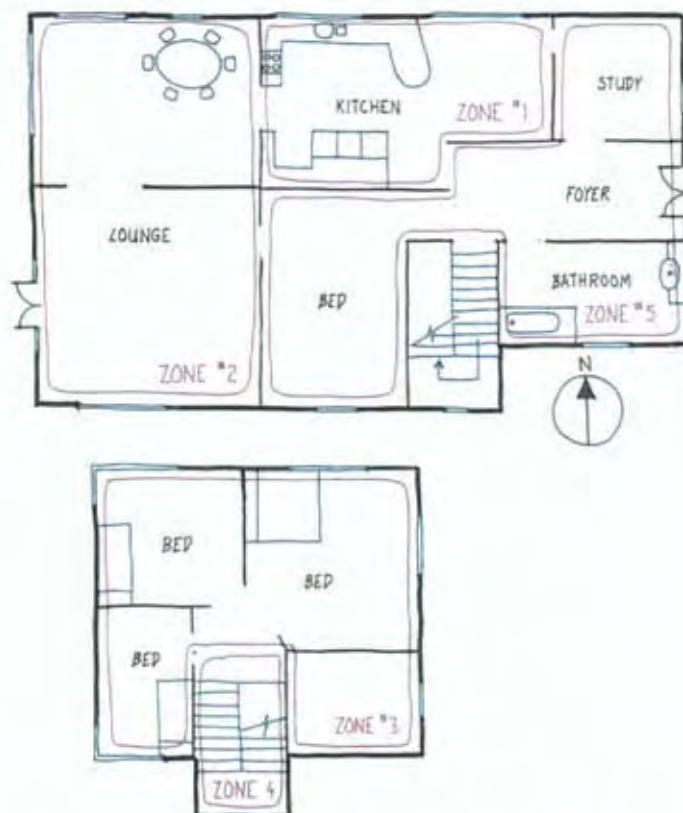
Figure 3: Schematic of the large house. The total floor area is 245 m 2 . The lounge/dining, kitchen and upper storey bedroom were considered to be the most important rooms in terms of overheating. The house is modelled as having seven different temperature zones (including two roof spaces).
