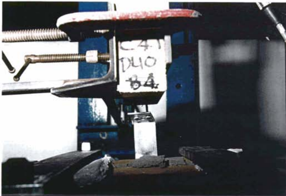
Photograph 8: Type 2 tie after axial cycling, showing nail withdrawal due to 'levering' action during compression
