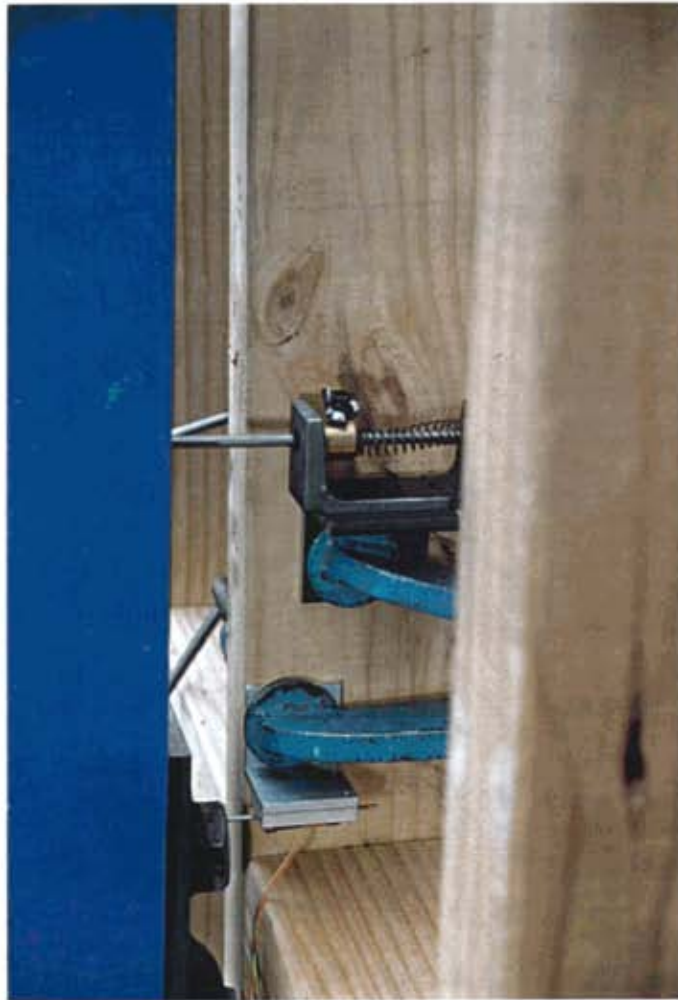
Photograph 13: Monitoring stud movement under tie installation
