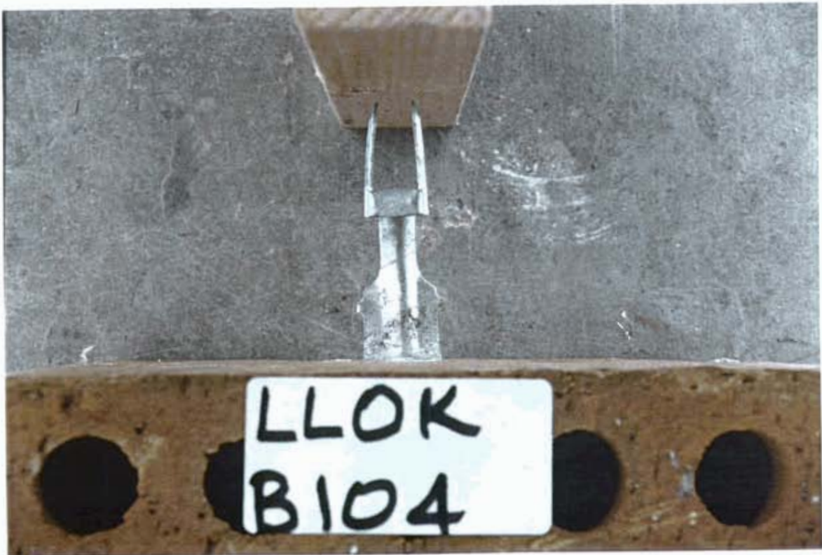
Photograph 9: Type 3 tie after axial cycling showing nail withdrawal
