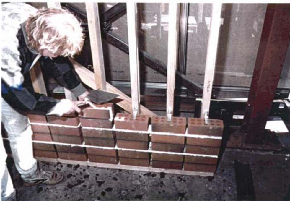
Photograph 2: Construction of series 1 specimens
