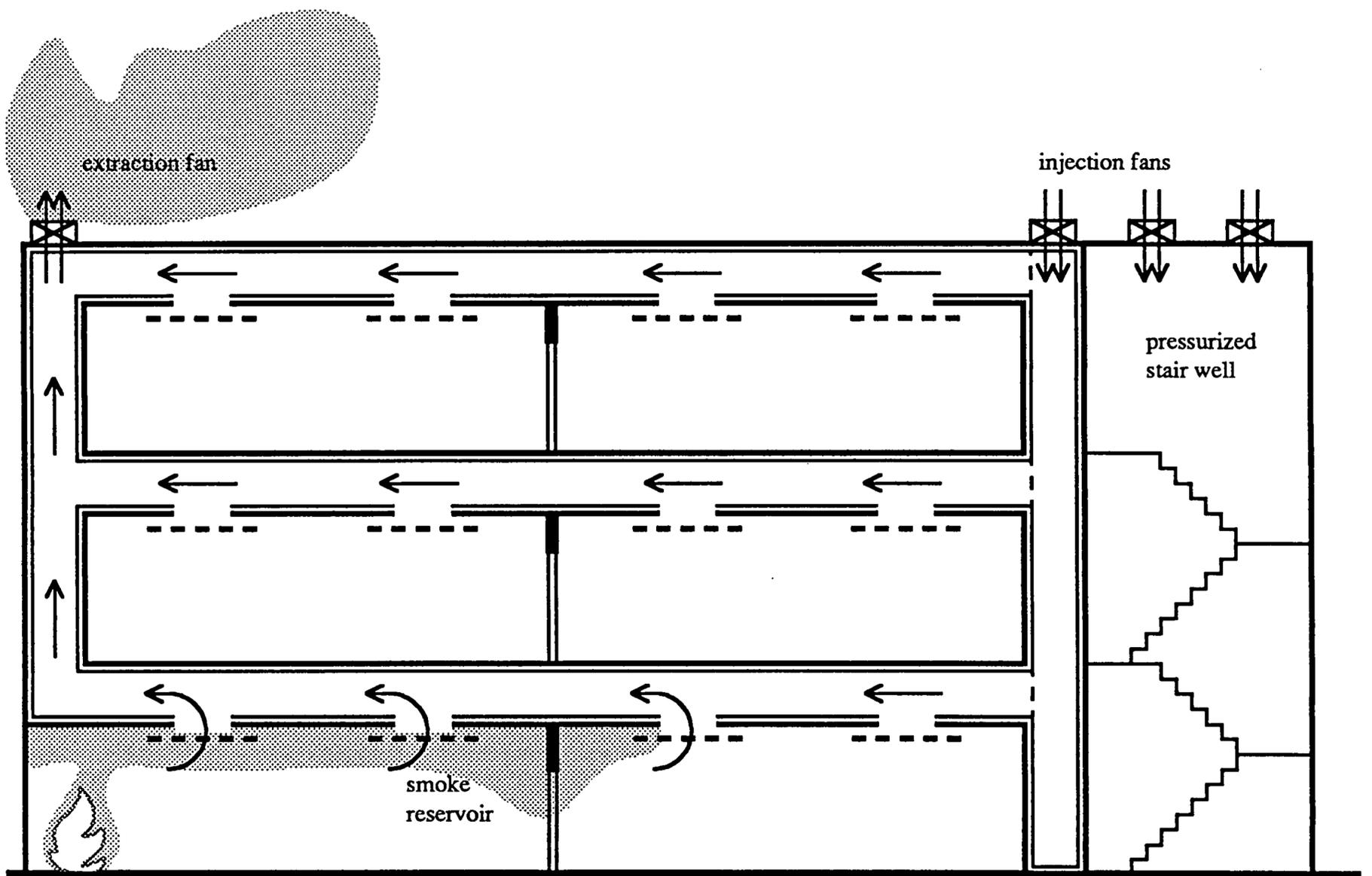
Figure 2 (a) Smoke reservoirs in a compartmented building
