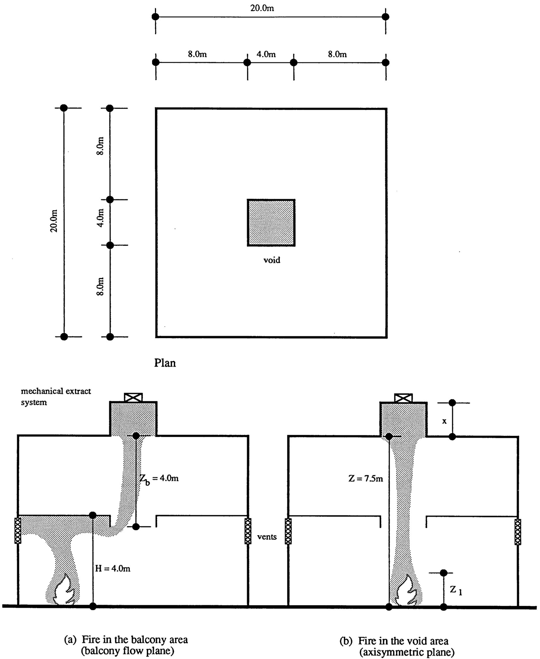
Figure 10 Plan and elevation of sample building used for smoke extraction calculations.
