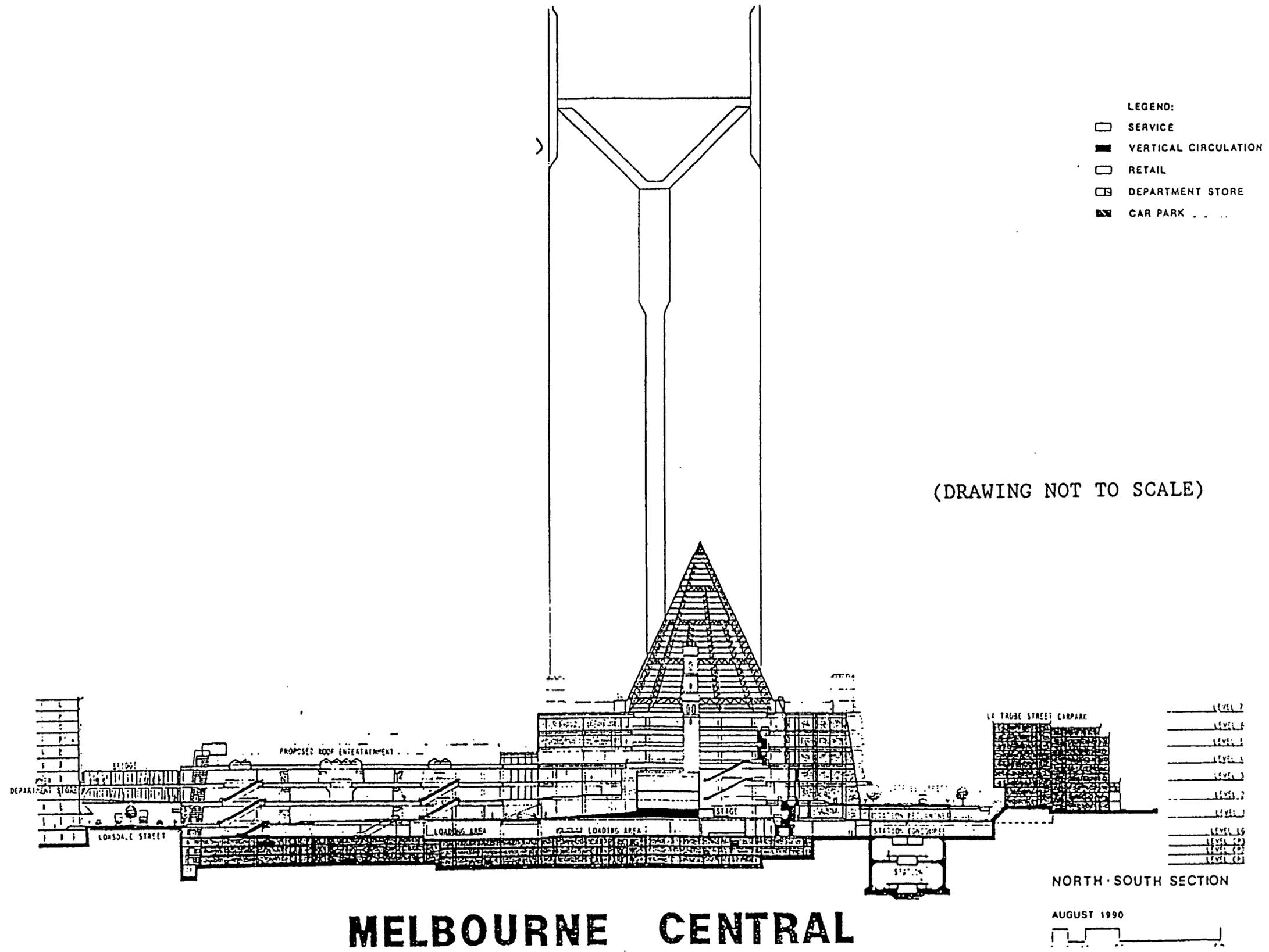
Figure 8 Elevation of the Melbourne Central Complex showing the atrium cone and the outline of the 56-storey office building in the background
