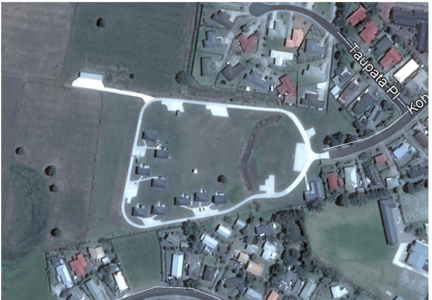
ABOVE: Early site plan showing the first two stages of development for He Korowai Trust, and aerial imagery showing the completion of the first nine houses (Stage 1). The layout of the kāinga includes a one-way driveway around the periphery of the site, leaving space in the centre of the site for Tamariki to play safely, away from car traffic.
