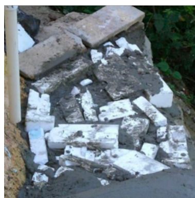
Figure 10 - Polystyrene contaminated by concrete. (ClevaCo, 2023).
