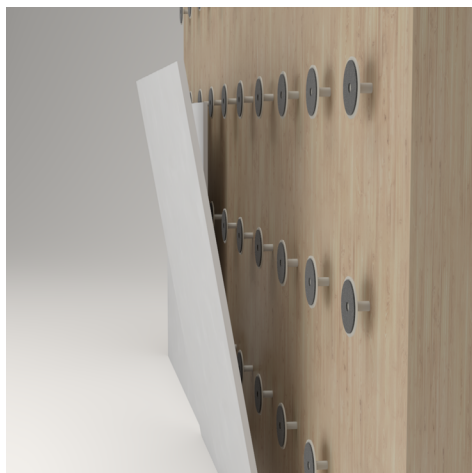
Figure 31 - StoSystain R Grip fixing system. The mechanical fixation element is round shaped (rotunda) with a hook fastener and has a screw thread for adjusting the irregularities in the load-bearing wall by moving the façade panel forward and backwards. (Oswald, 2024)
