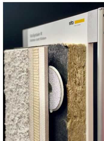
Figure 31 - StoSystain R Grip fixing system. The mechanical fixation element is round shaped (rotunda) with a hook fastener and has a screw thread for adjusting the irregularities in the load-bearing wall by moving the façade panel forward and backwards. (Oswald, 2024)
