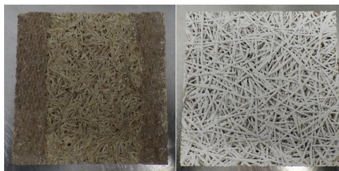
Figure 3: Representative 19 mm fine fissured mineral tile layer specimen (Exposed face on left, adhered face on right)
