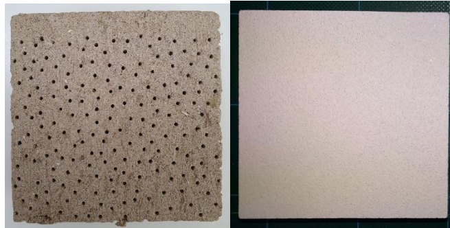
Figure 4: Representative dB Acoustic mineral tile layer specimens (24 mm perforated unpainted on left, FH6933 30 mm painted on right)
