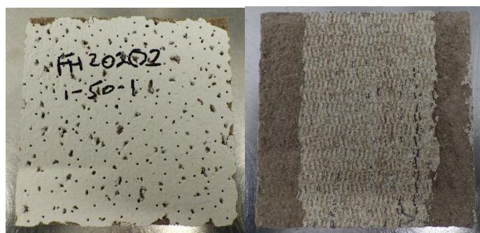
Figure 3: Representative 19 mm fine fissured mineral tile layer specimen (Exposed face on left, adhered face on right)
