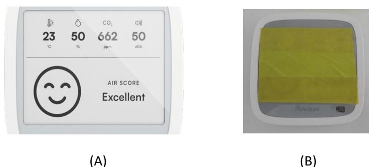
Picture 1: Air quality monitor display (A) and with masking tape applied to cover the screen (B)
