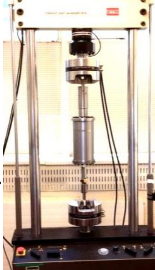
Figure 36: Force-displacement of the 2-4 D3 device with 3 orifices open when providing damping force under sinusoidal input loading with different frequencies and an input amplitude 35 mm. The experimental test setup in the MTS-810 machine.
