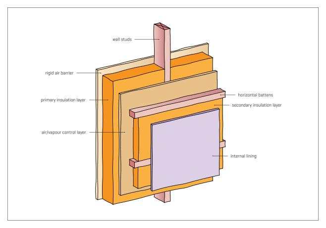
Figure 2. A 45 mm thick interior batten fixed over an air/vapour control layer creates space for a secondary insulated cavity.
