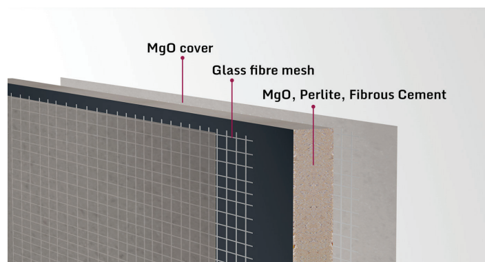
Typical structure of a magnesium oxide (MgO) board.
