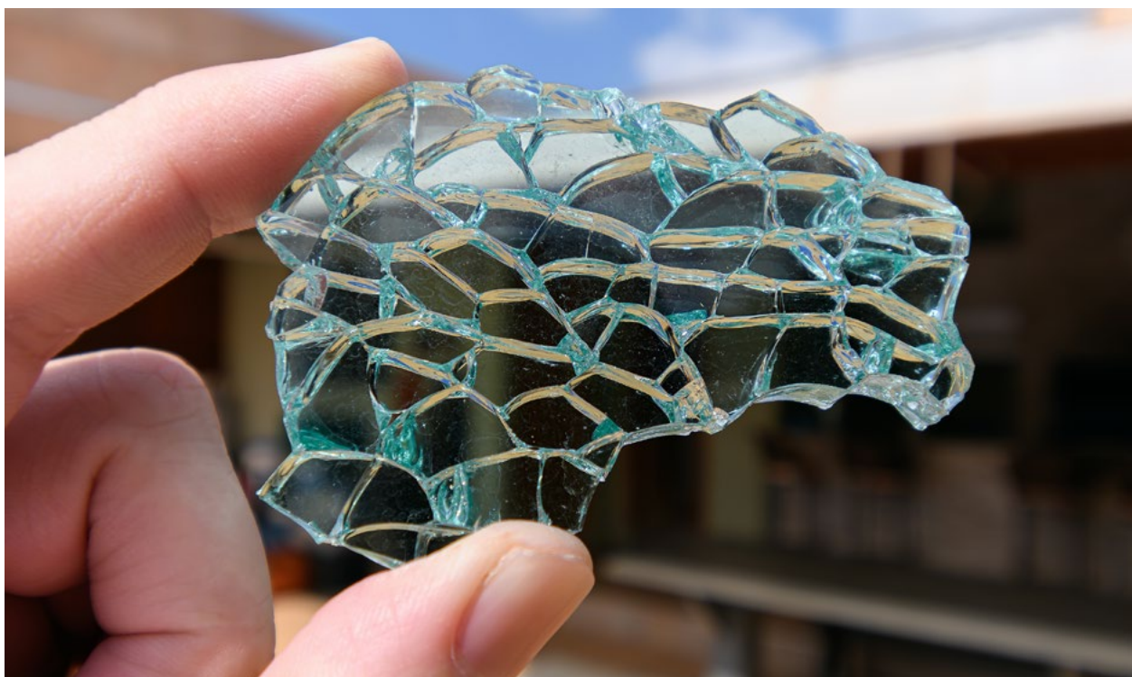
When toughened glass is broken, it shatters into tiny pieces, vastly reducing the danger of injury from flying shards of glass with sharp edges.
