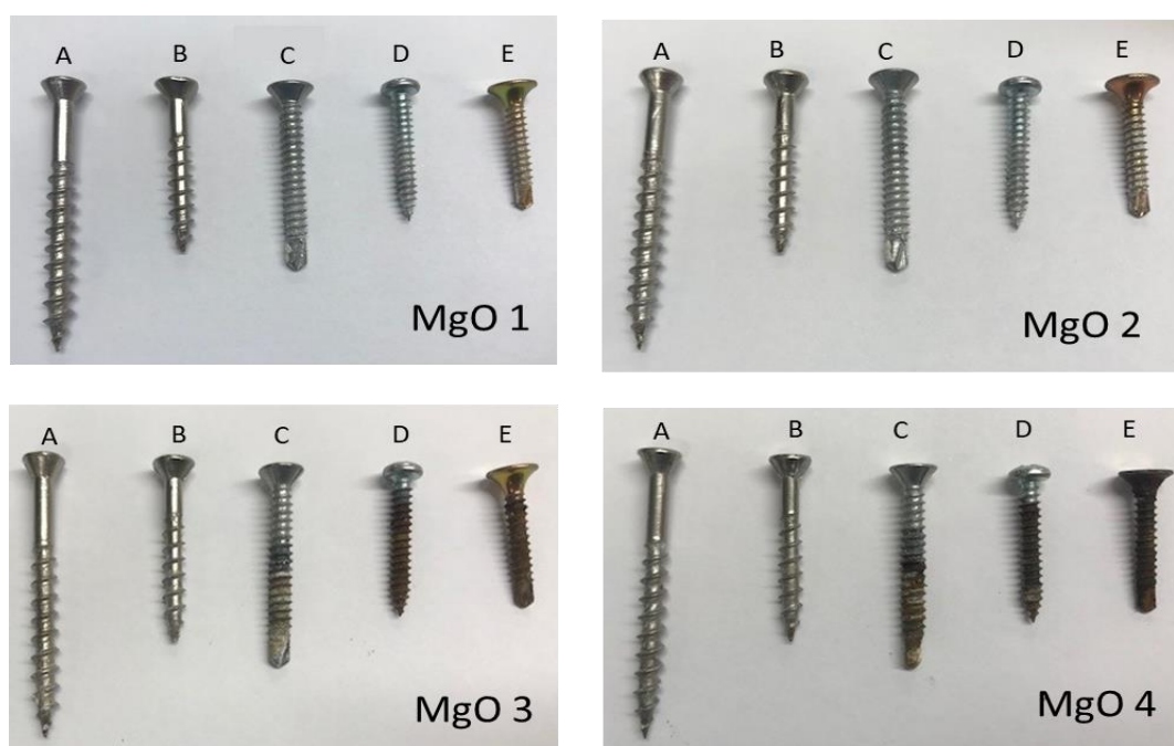
Figure 8. Conditions of screws attached to samples parallel to the sample surface (A) 316 stainless steel, (B) 304 stainless steel, (C) mechanically plated, (D) electroplated, (E) passivated electroplated.
