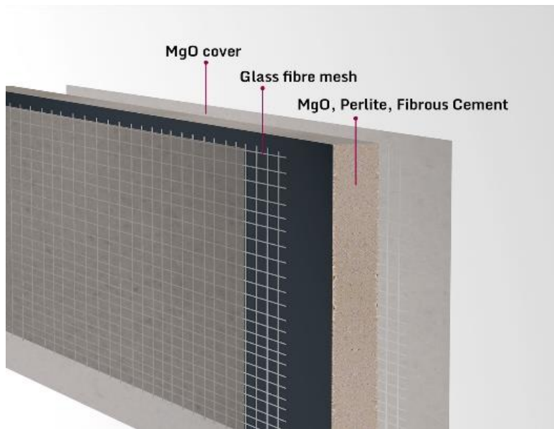
Figure 1. Structure of a typical MgO board.
