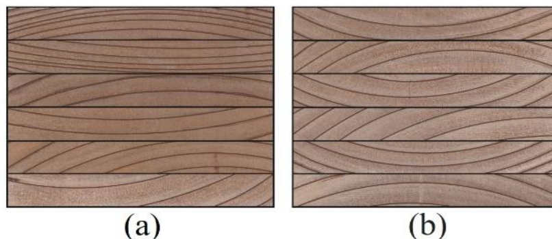
Figure 2. Annular ring arrangements: (a) alternating annular ring orientation with pith side of outermost laminations facing inwards; (b) limited alternation in annular ring orientation with pith side the outermost laminations facing outwards.
