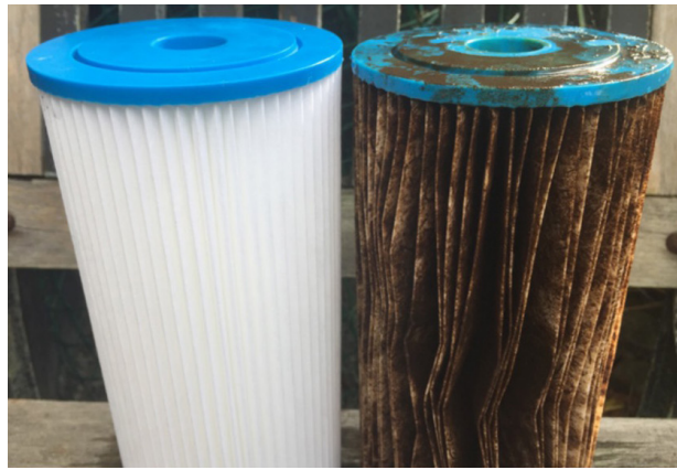
Figure 5. A new pleated mesh cartridge filter and the used filter it is replacing. Filters should be replaced regularly in line with the manufacturer's instructions.
