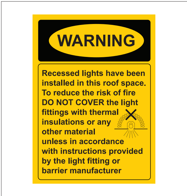
Figure 4. Example of a warning sign required in an accessible roof space.
