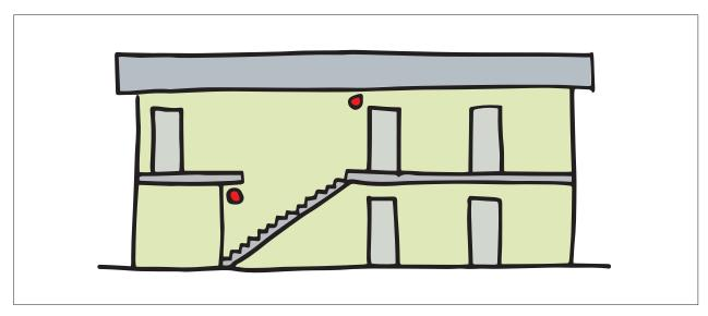
Figure 6. Where a house has more than 1 storey, there should be a smoke alarm on each level.
