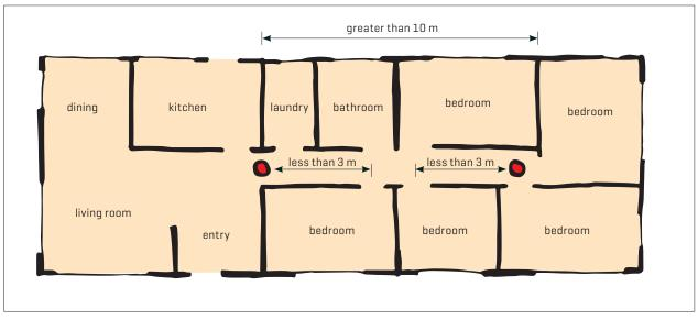
Figure 4. Two smoke alarms are needed in extended plan houses. A smoke alarm must be within 3 m of each bedroom door.
