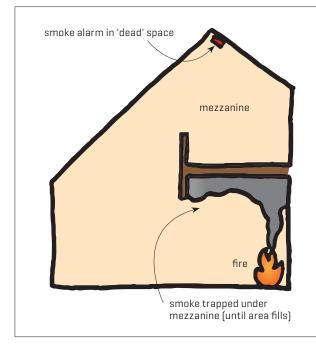
Figure 1. Example of a smoke alarm located in a dead space.
