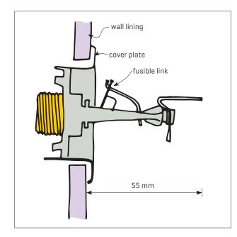
Figure 10. Horizontal sidewall sprinkler head.
