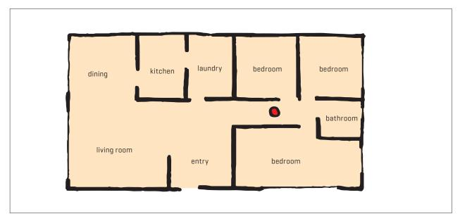
Figure 3. A smoke alarm in a small dwelling should be placed between the sleeping area and living area.
