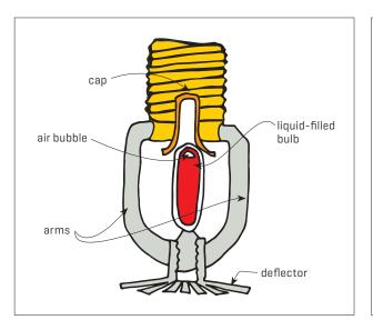
Figure 8. Glass bulb type sprinkler.
