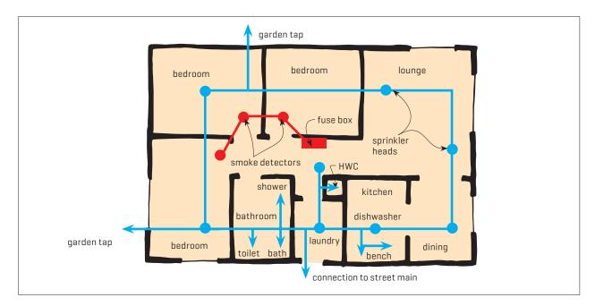
Figure 11. Cold water supply loop and interconnected and hard-wired smoke detection system.
