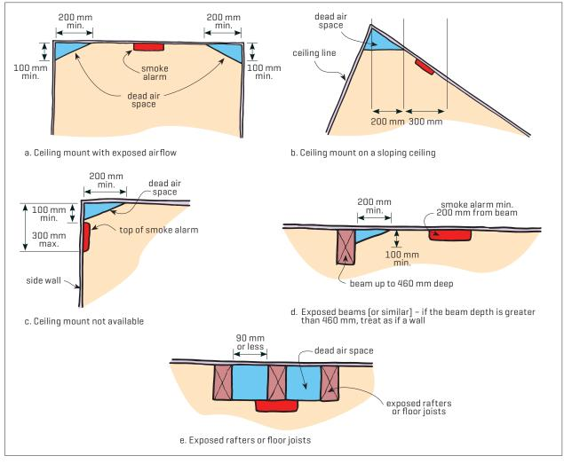
Figure 7. Acceptable locations for smoke alarms to ensure proper operation as per NZS 4514:2009.
